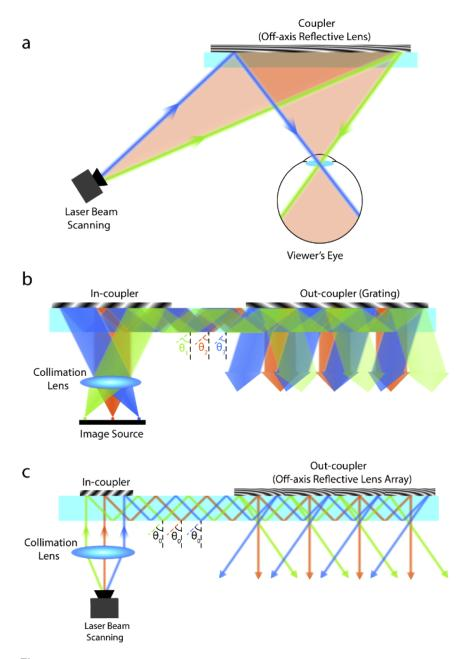
**Fig. 1.** Schematic diagram of different see-through display systems: (a) Retinal scanning display with a scanning laser beam and an off-axis combiner lens. (b) Traditional waveguide display with light paths of three pixels. The propagation angle in the waveguide is different for each pixel. (c) Our proposed scanning waveguide display with illustration of light paths of three pixels. The propagation angle in the waveguide is fixed for all pixels.
