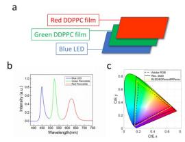
**Figure 4.** Application of the ultra-stable perovskitepolymer composite films as a) downconverting sheet in display backlighting. b) Emission spectra of a white LED system with green CsPbBr<sub>3</sub> DDPPC and red DDPPC films as downconverters for blue LEDs. c) Color gamut coverage of the white LED systems with Adobe RGB and Rec. 2020 standards for comparison in CIE 1931.
