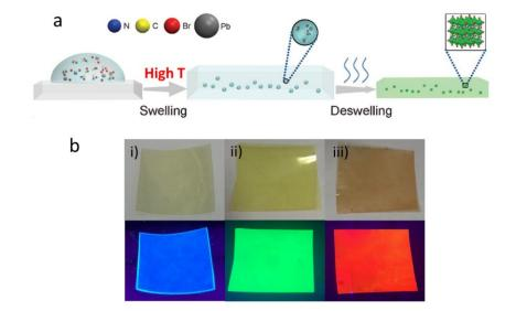
**Figure 1.** a) Scheme of ultrastable perovskite-polymer composite formation process through deep-dyeing swelling-deswelling microencapsulation strategy. b) Images of ultrastable perovskite-polymer composite films of different colors under ambient light (upper) and 395nm UV light (lower) excitation. Perovskite precursor compositions are i) CsPbCl<sub>1</sub>Br<sub>2</sub>, ii) CsPbBr<sub>3</sub>, iii) CsPbBr<sub>0.75</sub>I<sub>2.25</sub>.
