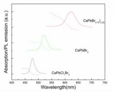
**Figure 2.** UV-vis(dotted line) and PL emission(solid line) for the CsPbX<sub>3</sub> DDPPC film spectra.
