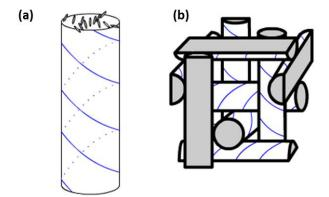
When no voltage is applied, BPLC appears optically isotropic with refractive indices being the same in all directions  $n_i$ . As an electric field is applied, birefringence is induced along the direction of electric field. The induced birefringence  $\Delta n_{ind}$  can be described by the Kerr effect in the low field region:
