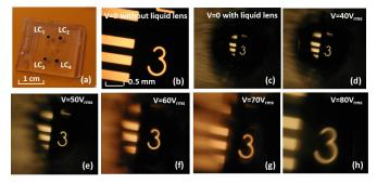
Fig. 2. (a) Lens cell, (b) the images observed through the microscope without the liquid lens at V = 0, and (d)-(k) with the liquid lens at the specified voltages (Media 1).
