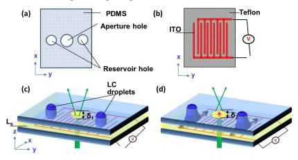
Fig. 1. (a) The layout of lens hole and reservoir holes on the top acrylic slab, (b) the layout of the interdigitated ITO electrode and Teflon layer on the bottom glass slab (the aperture and width of ITO stripes are not drawn by scale.), (c) liquid lens and LC pistons are at rest state, and (d) liquid lens is actuated by LC pistons.
