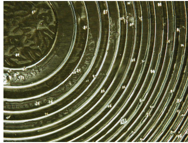
Fig. 3. Microscope images of the PSCOF Fresnel lens cell at V = 0 . The sample is sandwiched between crossed polarizers.
