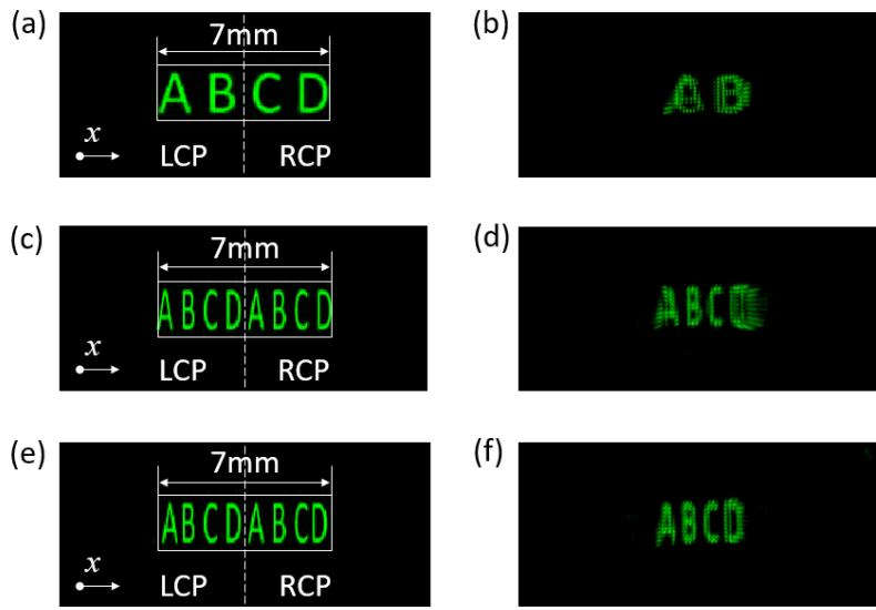
Fig. 11. (a), (c), (e) Input image contents during the rendering and (b), (d), (f) the corresponding imaging results.
