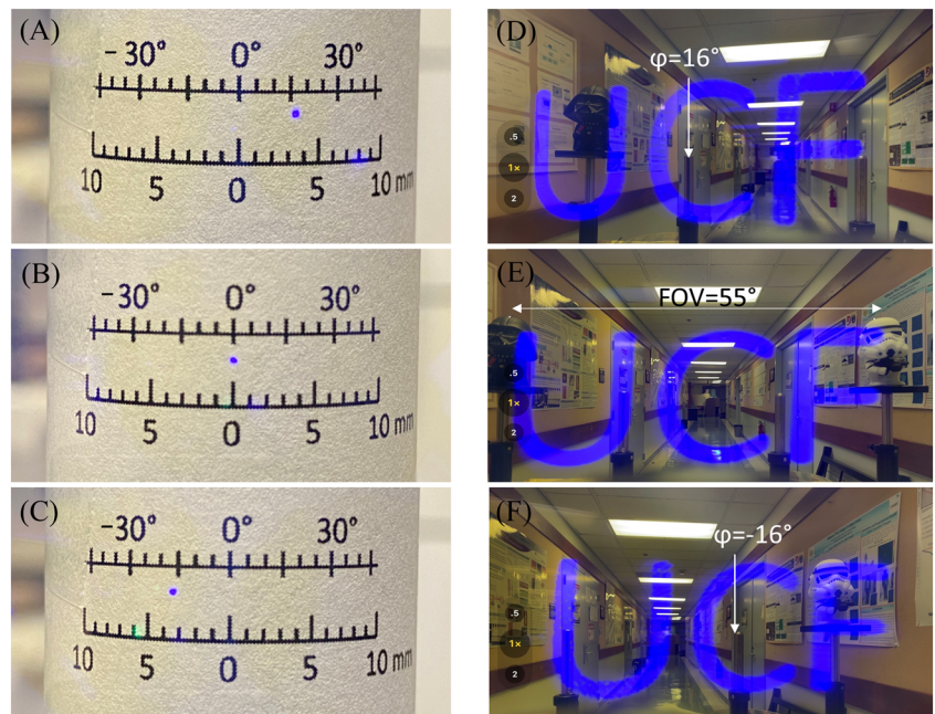
FIGURE 8 (A–C) Photos of the focal point positions on the eyeball surface and (D–F) corresponding imaging results and gaze directions
