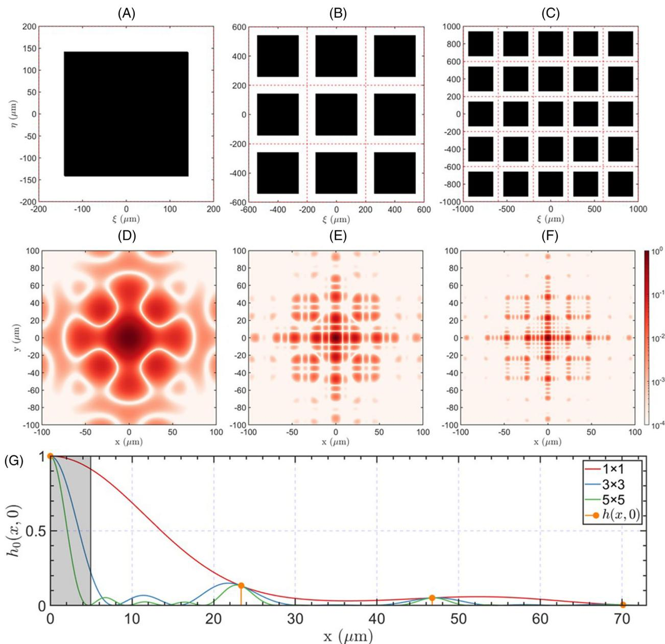
FIGURE 5 (A–C) With pixel size  $p = 400\ \mu\text{m}$  and aperture ratio  $\alpha = 50\%$ , unit cell functions  $t_0(\xi, \eta)$  with  $1 \times 1$ ,  $3 \times 3$ ,  $5 \times 5$  pixels in one unit cell for conventional pixel structures. (D–F) Fourier transforms (FTs) of unit cell functions in (A)–(C). (G) The horizontal cross-section  $h_0(x, y)$  excerpted from (D)–(F)
