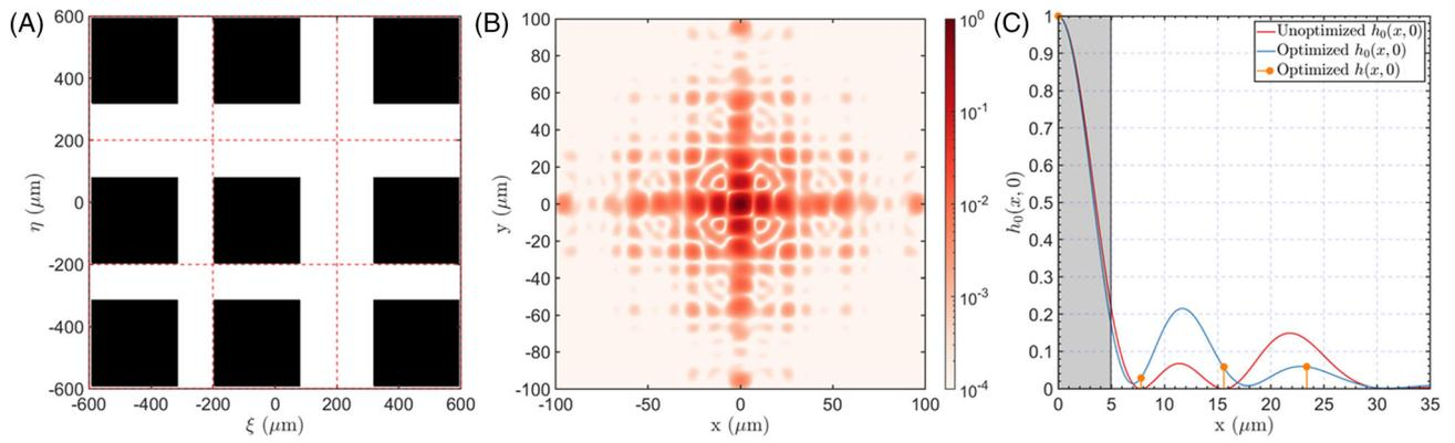
**FIGURE 7** (A) An optimized pixel structures within a unit cell with  $3 \times 3$ -pixel size and aperture ratio  $\alpha = 50\%$ . (B) Fourier transform (FT) of the optimized structure. (C) Horizontal cross section  $h_0(x,0)$  of the optimized and unoptimized structures and PSF  $h(x,0)$  of the optimized structure
