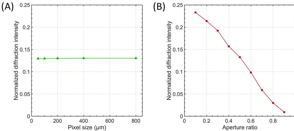
**FIGURE 4** (A) At aperture ratio  $\alpha = 50\%$ , the relative diffraction intensity is invariant to the pixel size  $p = 50\text{--}800\ \mu\text{m}$ . (B) With pixel size  $p = 400\ \mu\text{m}$ , the relative diffraction intensity decreases as aperture ratio  $\alpha$  increases from 10% to 90%
