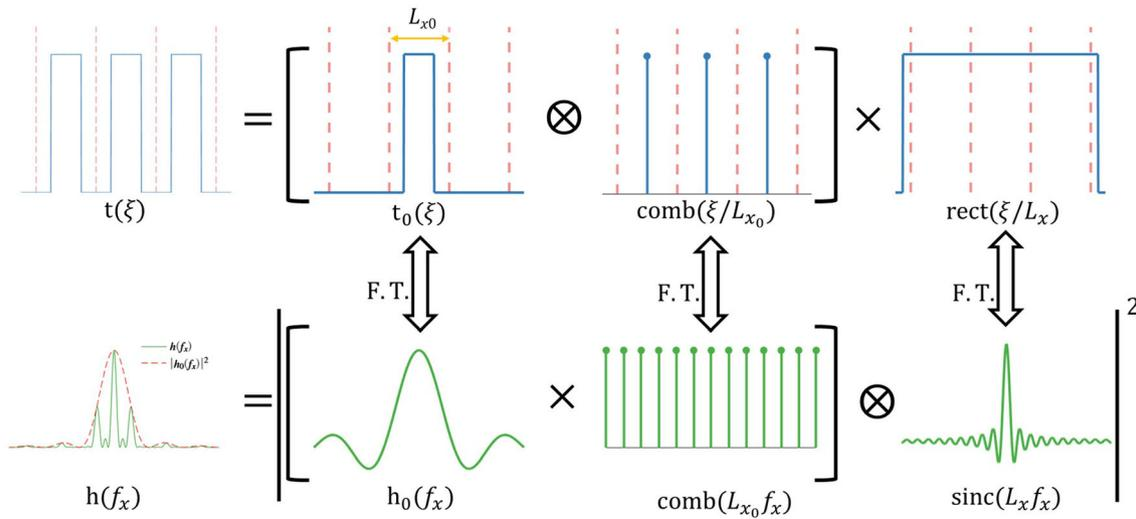
**FIGURE 3** A visual representation of point spread function (PSF) calculation in an imaging system including a transparent display. For simplicity, 1D derivation is shown here but it is easy to extend to two dimensions
