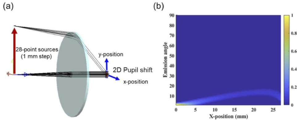
**Fig. 3.** (a) Schematic of Fresnel VR system in LightTools. (b) Simulated angular power collection efficiency of the 28-point source in an VR system.
