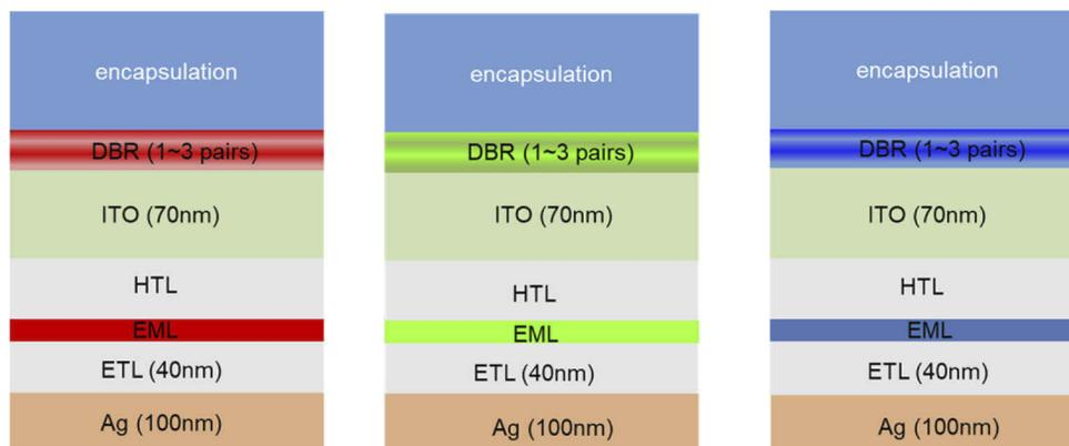
**Fig. 5.** Layer structure of RGB OLED devices.
