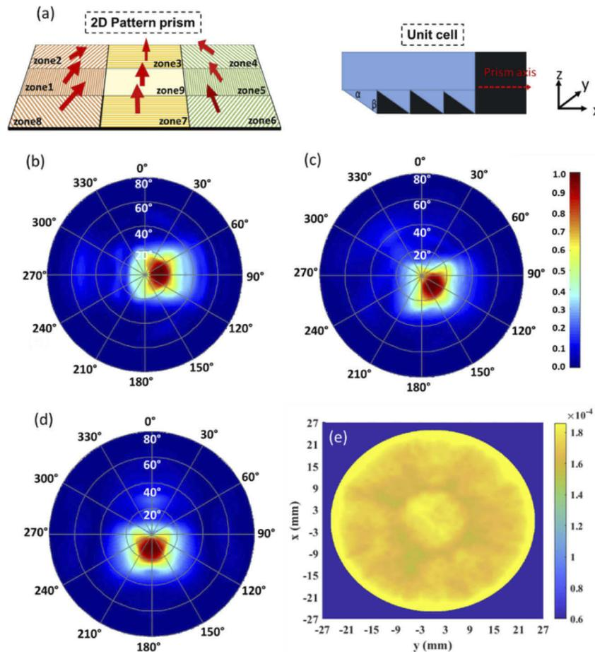
**Fig. 11.** (a) Schematic of the 2D patterned prism. The backlight radiation pattern in local (b) zone 1, (c) zone 2, and (d) zone 3. (e) The TLE distribution of each pixel in an LCD-based VR system with 2D patterned prism. BEF:  $n = 1.7$ .
