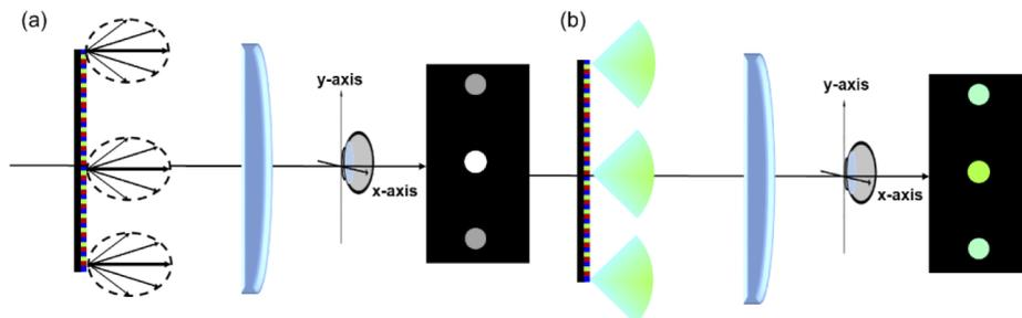
**Fig. 2.** Schematic of (a) field brightness non-uniformity and (b) field color non-uniformity in VR. According to the pixel position (top, center, and down), three circles on the right of the figure represent the image received by the eye, respectively.
