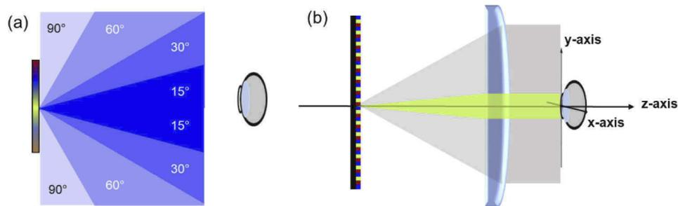
**Fig. 1.** Schematic of (a) direct-view display, and (b) VR display system consisting of a display panel, eyepiece, and eye pupil.
