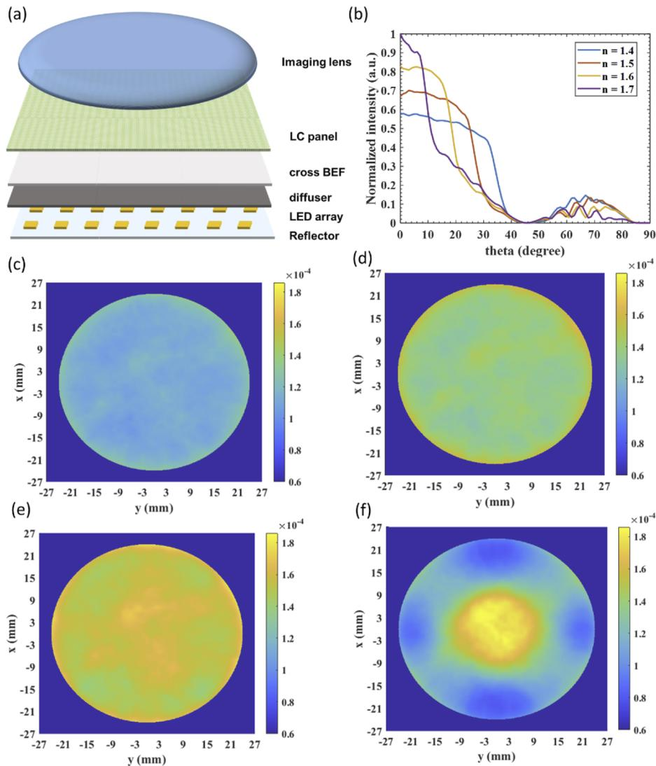
**Fig. 10.** (a) Schematic of the LCD based VR system. (b) The angular intensity distribution of backlight unit with BEF ( $n = 1.4$  to  $n = 1.7$ ). The TLE distribution of each pixel in the LCD based VR system with BEF having various refractive index: (c)  $n = 1.4$ , (d)  $n = 1.5$ , (e)  $n = 1.6$ , and (f)  $n = 1.7$ .
