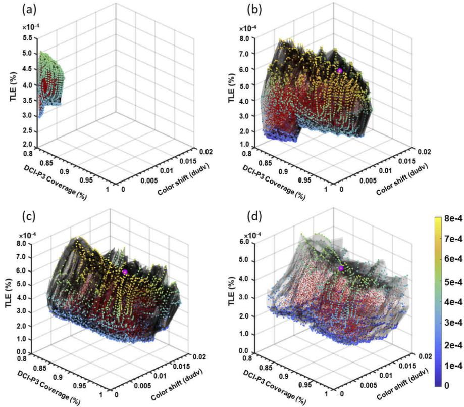
**Fig. 8.** The optimization results of RGB OLED displays: (a) without DBR (b) with 1 pair of DBR, (c) with 2 pairs of DBR, and (d) with 3 pairs of DBR in an VR system. Three objectives are considered simultaneously. (Magenta point: optimal solution)
