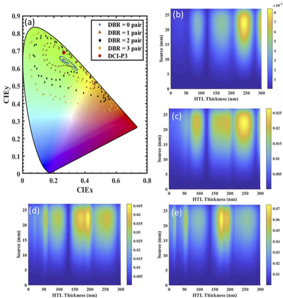
**Fig. 7.** (a) Simulated field color coordinate (CIE1931) of the green OLED in the VR system. Simulated field color non-uniformity of the green OLED devices: (b) without DBR, (c) with 1 pair DBR, (d) with 2 pairs of DBR, and (e) with 3 pairs of DBR.
