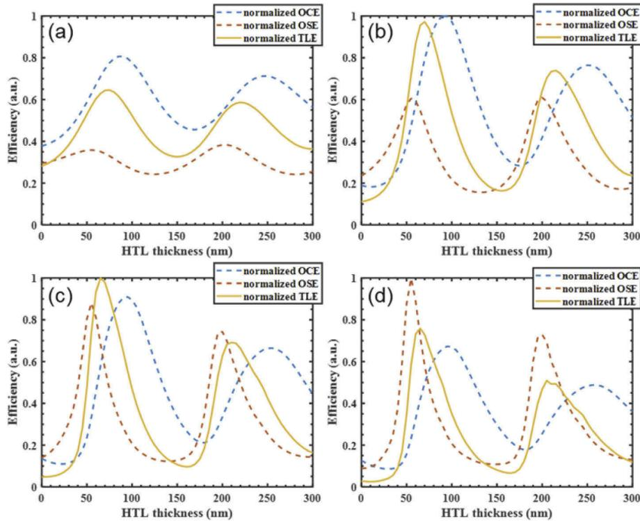
**Fig. 6.** The simulated OCE, OSE, and TLE of the green OLED device: (a) without DBR, (b) with 1 pair of DBR, (c) with 2 pairs of DBR, and (d) with 3 pairs of DBR.
