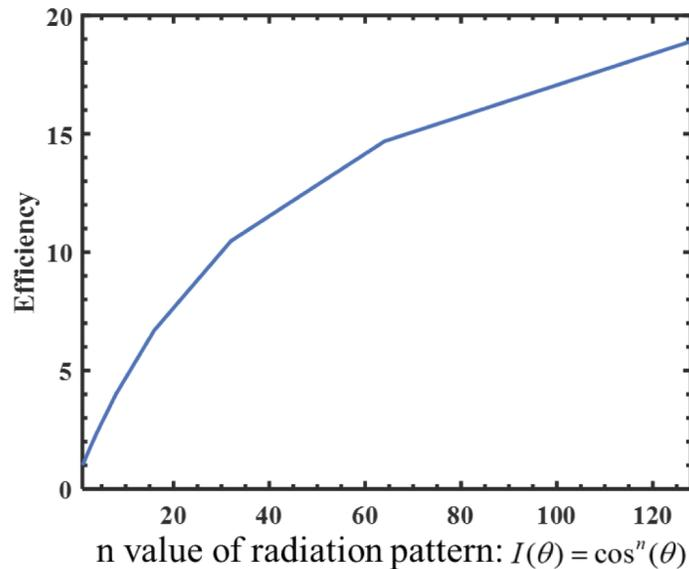
**Fig. 4.** Normalized OSE of a display with various radiation pattern in a VR system.
