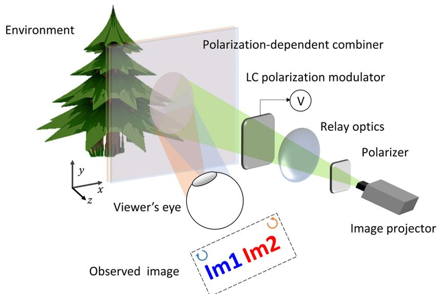
of the two polarization paths. This area can be further enlarged when the eye relief is decreased, the size of the intermediate image is increased, or the divergence angle of the two paths is reduced.
