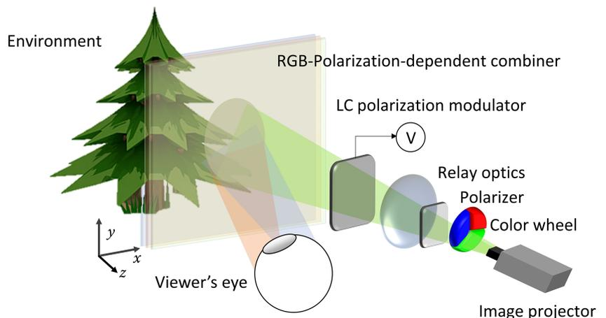
FIGURE 8 Schematic illustration of the RGB system
