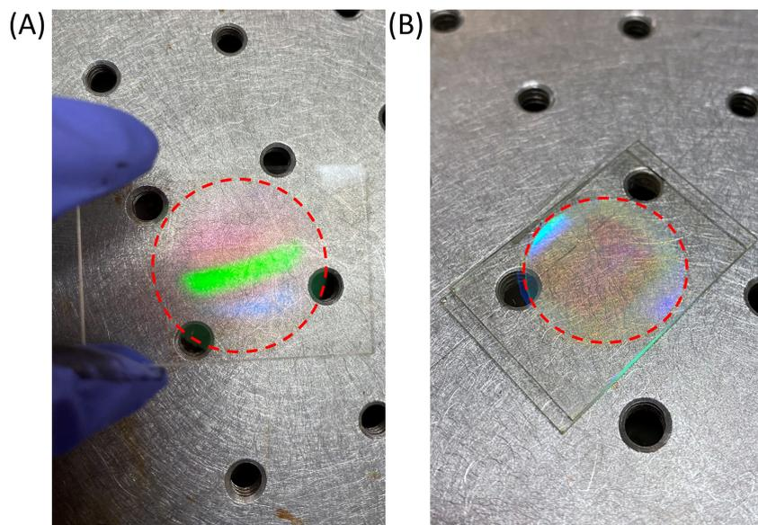
FIGURE 4 Photo of (A) the PVL-L and (B) the PDC consisting of PVL-L and PVL-R
