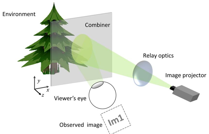
**FIGURE 3** Schematic illustration of the polarization-time multiplexing free space AR system
