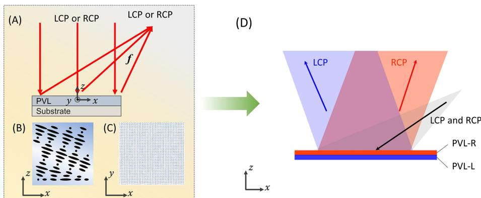
**FIGURE 1** Schematic illustrations of (A) a PVL with (B) surface alignment and (C) CLCs structure. (D) Schematic diagram of the PDC with two cascaded PVLs
