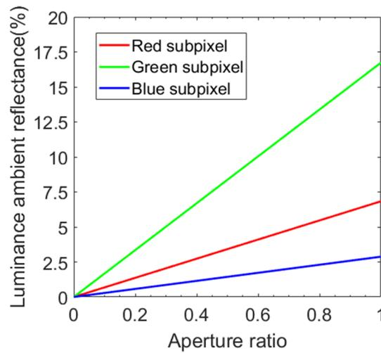
**Figure 8.** The luminance ambient reflectance of RGB subpixels in color-conversion micro-LED display at different aperture ratio.
