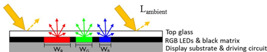
**Figure 1.** Device structure of our proposed RGB micro-LED display.
