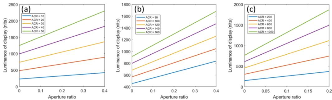
**Figure 9.** The required luminance of color-conversion micro-LED display as a function of aperture ratio for achieving the listed ACR under three ambient light illuminances: (a) 2000 lux, (b) 450 lux and (c) 200 lux.
