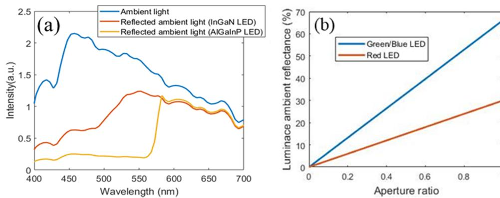
**Figure 2.** (a) The intensity spectrum of ambient light, ambient light reflected by AlGaInP based LED, and ambient light reflected by InGaN based LED. (b) The luminance ambient reflectance of RGB micro-LEDs at different LED chip aperture ratio.
