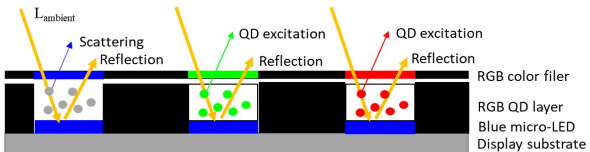
**Figure 5.** Device structure of our color-converted micro-LED display.
