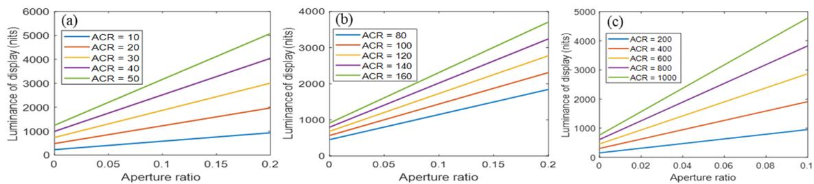
**Figure 3.** The required luminance of display, as a function of aperture ratio, for achieving the listed ACR under three ambient light illuminances: (a) 2000 lux, (b) 450 lux, and (c) 200 lux.
