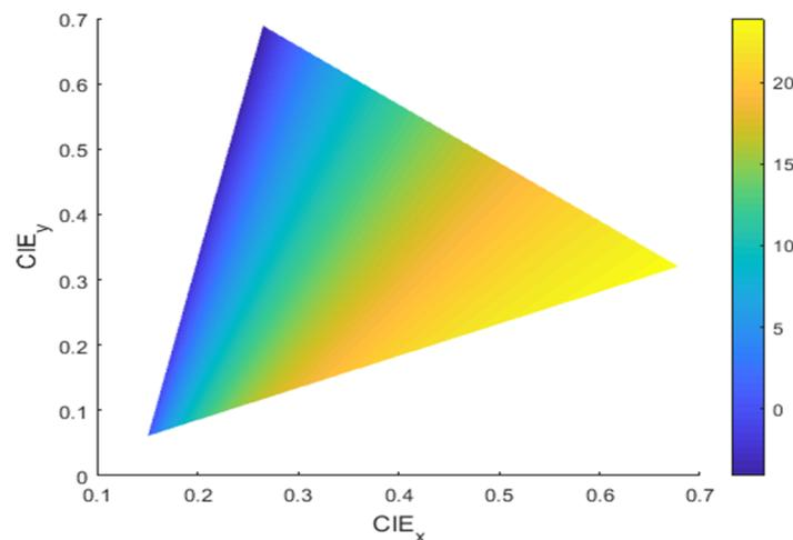
**Figure 14.** The decreased power consumption (unit: %) of RGB micro-LED displays with different chip sizes and uniform chip size.
