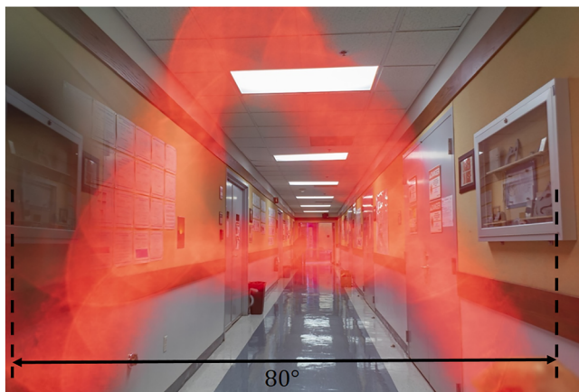
FIGURE 7 Photo of the see-through view with the display system presenting a letter “A.” The horizontal field of view is measured as 80°
