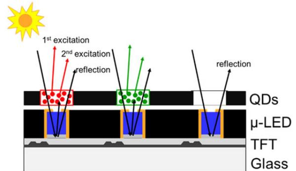
Figure 1. Device configuration of blue micro-LED array with red and green quantum dots as color conversion layer.
