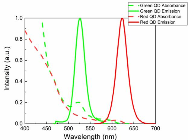
Figure 2. Absorbance and emission spectra of the employed green and red thick-shell quantum dots [11].
