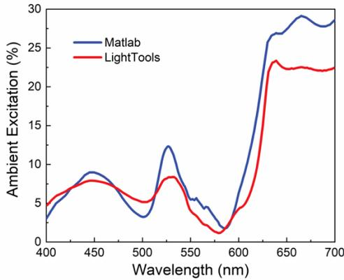
**Figure 6.** Calculated and simulated ambient light excitation spectra in QD-converted micro-LED displays with a top pixelated color filter based on Matlab and LightTools.
