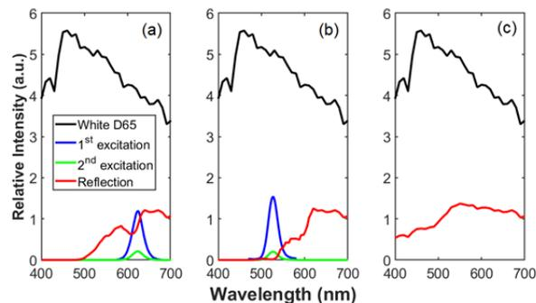
**Figure 4.** Calculated ambient light excitation and reflection for (a) red, (b) green and (c) blue subpixel in QD-converted full color micro-LED displays.
