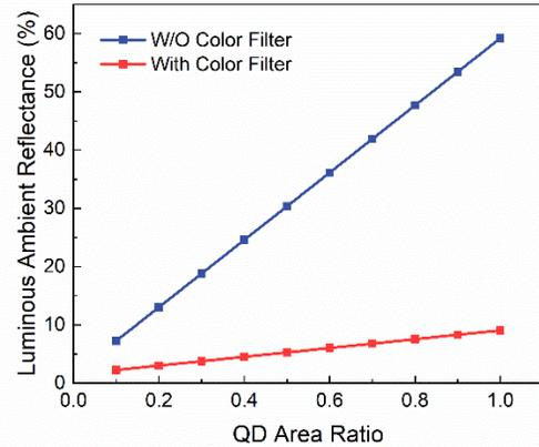
**Figure 8.** Calculated luminous ambient reflectance as a function of QD area ratio. The surface reflectance is 1.5%.
