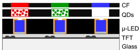
Figure 5. Schematic diagram for configuration of QD-converted micro-LED with top color filter.
