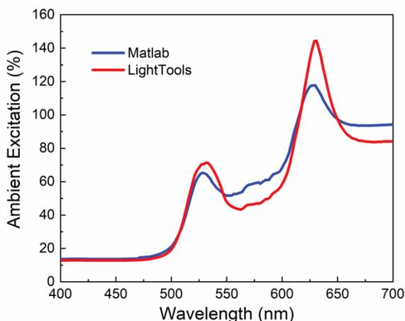
**Figure 3.** Calculated and simulated ambient light excitation spectra in quantum dot-converted micro-LED displays based on Matlab and LightTools.
