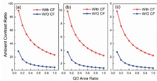
**Figure 9.** Calculated ambient contrast as a function of QD area ratio at ambient light of (a) 500 lux, (b) 5,000 lux and (c) 10,000 lux. The surface reflectance is 1.5%.
