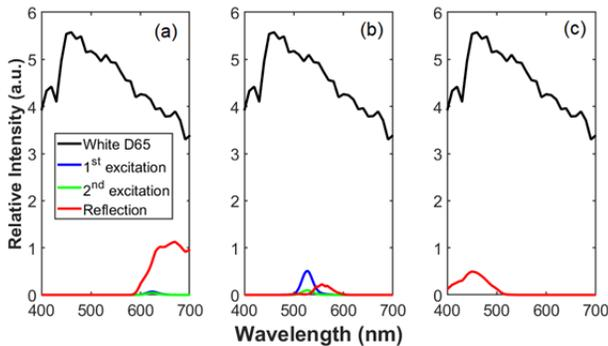
**Figure 7.** Calculated ambient light excitation and reflection for (a) red, (b) green and (c) blue subpixel in quantum dot-converted full color micro-LED displays with top color filter.
