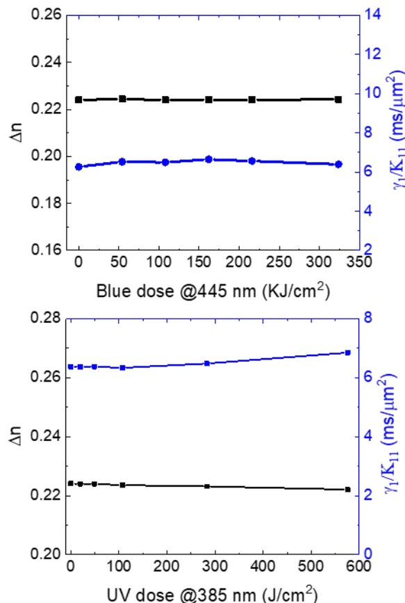
**Fig. 2.** (a) Measured blue-stability of UCF-2 exposed at 445 nm and  $40^\circ\text{C}$ . (b) Measured UV-stability of UCF-2 exposed at 385 nm. The probing laser beam is at  $\lambda=633 \text{ nm}$  and
