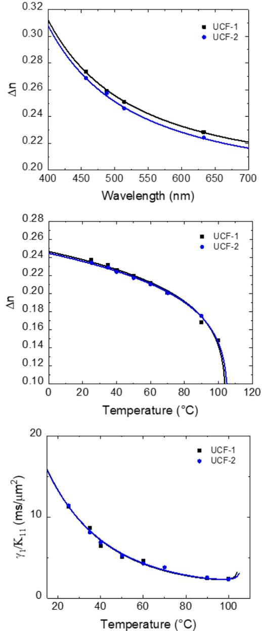
**Fig. 1.** (a) Temperature dependent birefringence at  $\lambda=633$  nm and 1 kHz. (b) Wavelength dependent birefringence at  $T=40^\circ\text{C}$ . (c) Temperature dependent visco-elastic coefficient at  $\lambda=633$  nm. Dots are experimental data and solid lines are fitting curves with Eqs. (1)-(3).
