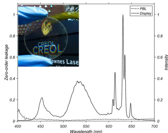
**Figure 7.** Measured zero-order leakage of the ultra-broadband PBL and the emission spectrum of the LCD displaying white light. Inside is a photo of the fabricated 2-inch PBL.
