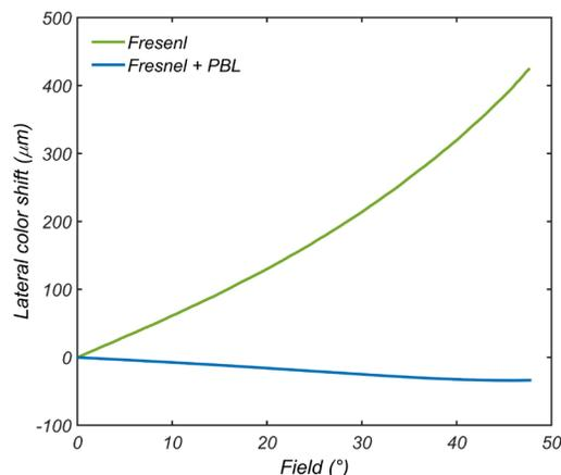
**Figure 6.** The lateral color shift of the VR viewing optics with and without PBL.
