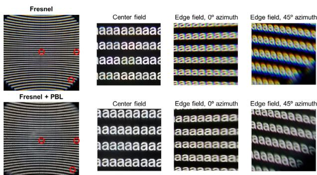
**Figure 9.** Full-field black-and-white image displayed on the LCD and the resulting images captured through the conventional and proposed hybrid viewing optics. The three enlarged parts are center field and edge fields at 0° and 45° azimuth from left to right.
