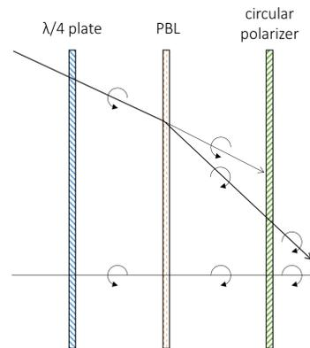
**Figure 4.** Illustration of polarization state changes through the planar optical parts in the proposed system.
