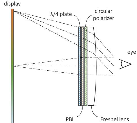
**Figure 3.** Optical layout of the proposed VR viewing optics.
