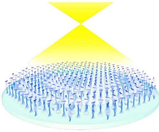
**Figure 2.** Schematic illustration of LC anisotropy axis orientation in the PBL with flat geometry and a twist-homo-twist structure for broadband operation.
