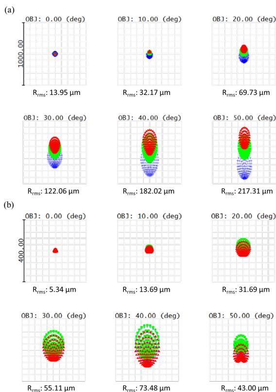
**Figure 5.** Standard spot diagram with RMS spot radius for (a) Fresnel singlet and (b) proposed hybrid optics. Color by wavelength, Red: 610nm, Green: 540nm, Blue: 450nm.
