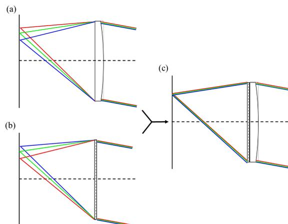
**Figure 1.** Illustration of transverse chromatic aberrations in a) a compact refractive Fresnel lens, b) a diffractive LC lens, and c) the proposed hybrid doublet exhibiting achromatic performance.
