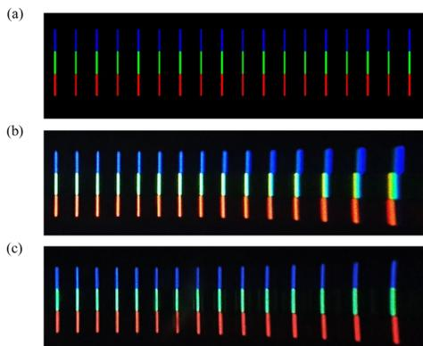
**Figure 8.** (a) Half-field CA testing pattern displayed on the LCD and the resulting images captured through the (b) conventional and (c) proposed viewing optics.
