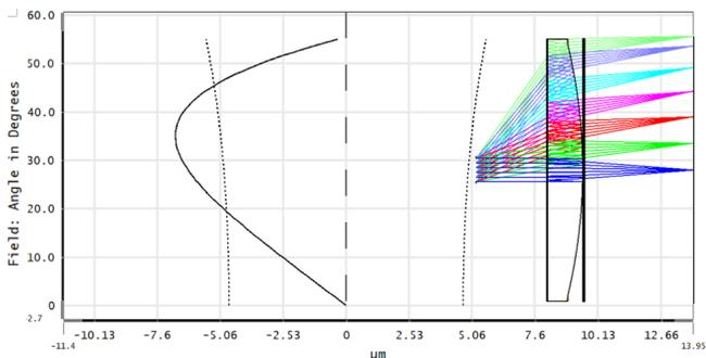
**Figure 10.** The lateral color shift of a pancake VR viewing optics with a PBL.
