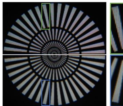
**Fig. 5.** Observed images from the near-eye display system without (upper) and with (lower) pixel density enhancement enabled by a PBD.
