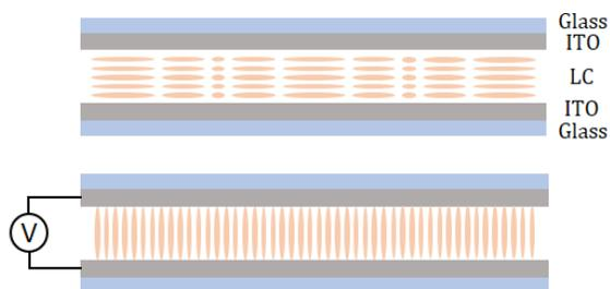
**Fig. 3.** Schematic illustration of PBOEs made of LCs sandwiched between transparent electrodes (upper) before and (lower) after dynamic switching.
