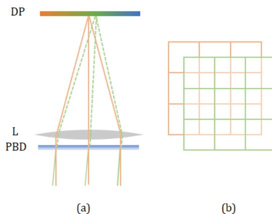
**Fig. 4.** (a) Schematic illustration of the optical system for pixel density enhancement with a PBD. (b) The generation of a half-pitch pixel grid by overlapping the original (orange) and shifted (green) pixel grid. (DP: display panel; L: magnifying lens.)
