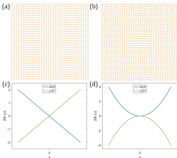
Fig. 1. Schematic distribution of LC anisotropy axis orientation in (a) a PB deflector and (b) a PB lens. The corresponding phase change of the (c) PBD and (d) PBL.
