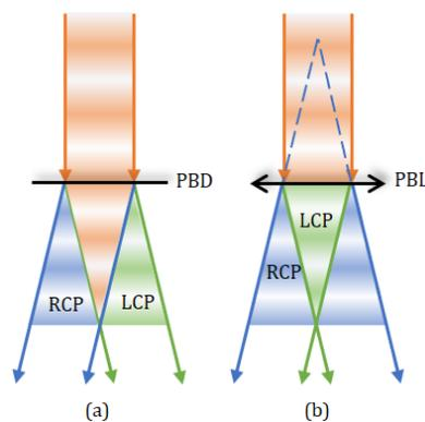
Fig. 2. Illustration of polarization dependency of PBOEs: (a) PBD diffracts RCP light to +1 order and LCP light to -1 order; (b) PBL serves as a diverging lens for input LCP light but a converging one for input RCP light.
