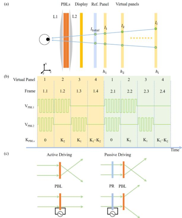
Fig. 7. (a) The principle of the additive light field display is illustrated with a stack of PBLs. Each virtual image panel, formed by a specific state of PBLs stack, generates independent additive light fields, which are merged into a single light field. (b) Time-multiplexing driving scheme of 4 additive virtual panels. (c) Illustration of active and passive driving modes of PBLs.
