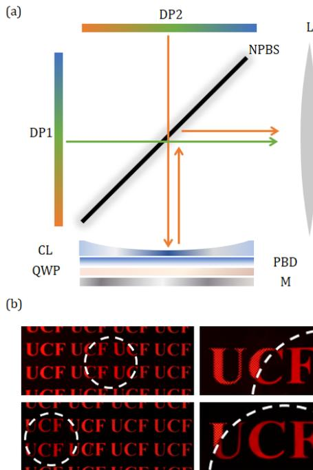
Fig. 6. (a) Schematic diagram of a foveated near-eye display system. (DP: display panel; NPBS: non-polarizing beam splitter; CL: concave lens; QWP: quarter-wave plate; M: Mirror; L: lens.) (b) Photography of foveated images from the near-eye display system before (upper) and after (lower) image shifting using a PBD.
