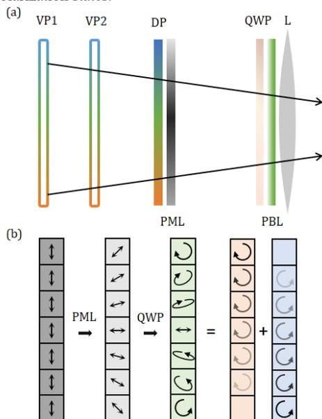
**Fig. 8.** (a) Schematic diagram of a polarization-multiplexed two-plane near-eye display system. (DP: display panel; VP: virtual plane; PML: polarization management layer; QWP: quarter-wave plate; L: lens.) (b) Schematic illustration of polarization state changes in the polarization multiplexed system.
