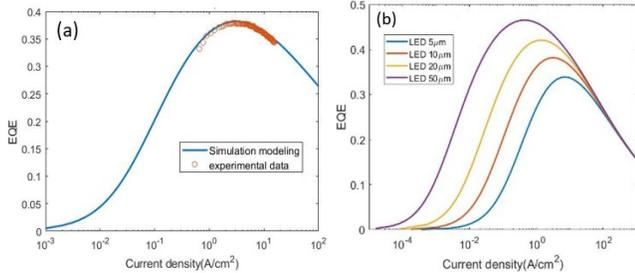
**Fig. 2.** (a) Measured EQE- $J$  curve and the fitted result. (b) Calculated EQE- $J$  curves for  $\mu$ LEDs with various sizes.
