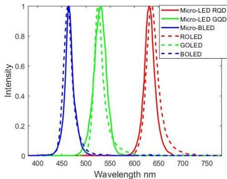
**Fig. 3.** Emission spectra of OLEDs and QD- $\mu$ LEDs.
