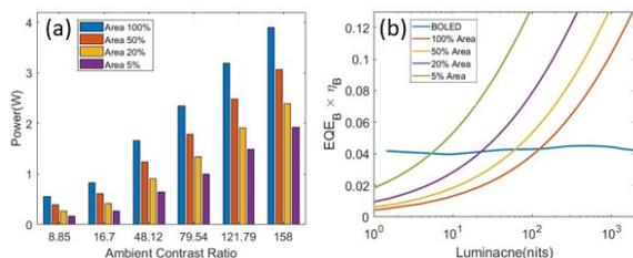
**Fig. 8.** The effect of current injection area on (a) power consumption of  $\mu$ LED (10 $\mu$ m) as a function of ACR; (b) The optical efficiency of blue OLED and blue  $\mu$ LED as a function of display luminance.
