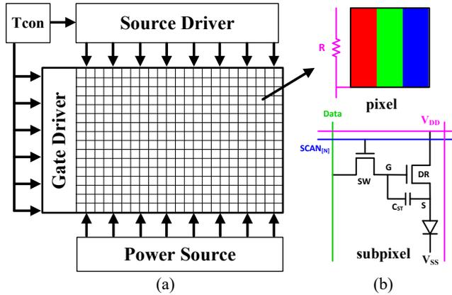
Fig. 5. (a) System diagram of AM displays. (b) Pixel diagram.
