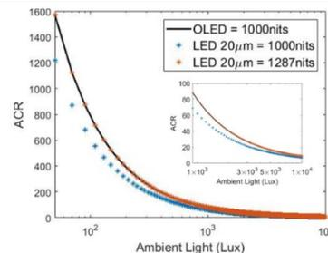
Fig. 1. ACR of OLED and  $\mu$ LED (20  $\mu$ m) with different display luminance.
