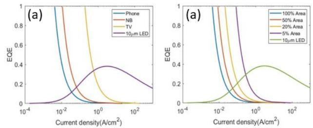
**Fig. 4.** (a) EQE- $J$  curves for different  $\beta$  values (corresponding to different applications) and for the  $\mu$ LED. (b) Effect of the current injection area on the driving range.
