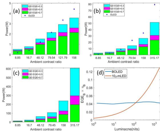
**Fig. 7.** The effect of QD efficiency on power consumption of (a) phone, (b) notebook, and (c) TV as a function of ACR (ambient light is 500 Lux and  $\mu$ LED is the optimized size in each application) (d) The optical efficiency of blue OLED vs. blue  $\mu$ LED at various luminance.
