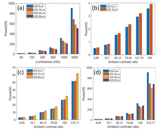
Fig. 6. Size effect of  $\mu$ LEDs on (a) power consumption of TV as a function of luminance and (b-d) power consumption as a function of ACR for (b) phone, (c) notebook, and (d) TV applications, where the illuminance of ambient light is 500 lux and the QD efficiency is 30%.
