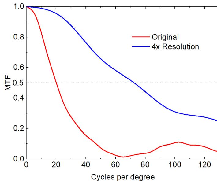
Fig. 6. The measured on-axis modulation transfer function for original and  $4 \times$  resolution in angular space. Note that the MTF drops to 0.5 at 20 cpd and 72 cpd for the original and  $4 \times$  resolution, respectively.
