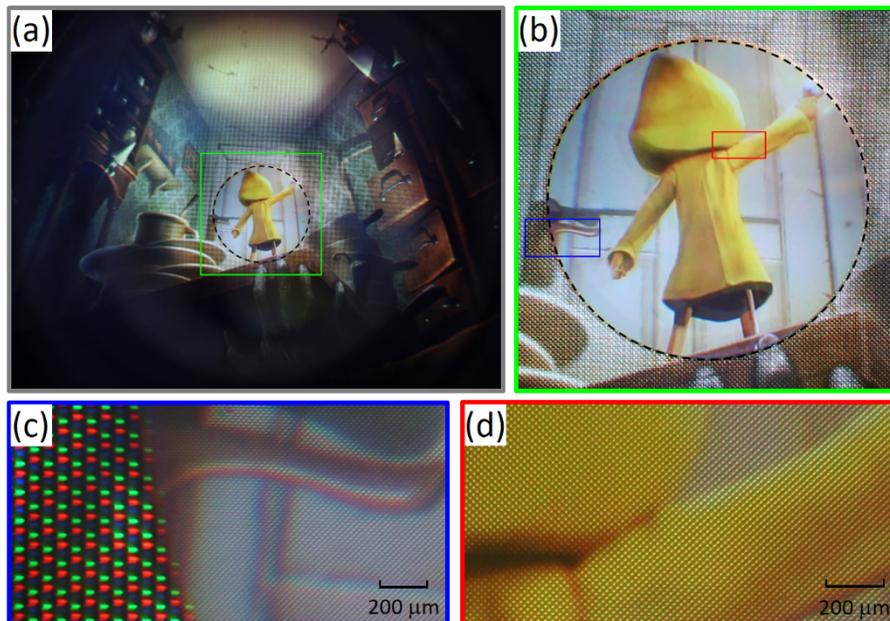
Fig. 5. The experimental photographs with the proposed multi-resolution foveated display with  $5 \times$  resolution enhancement: a) displayed image; b) the magnified green square region in (a); c) the magnified blue rectangle region in (b); d) the magnified red rectangle region in (b).
