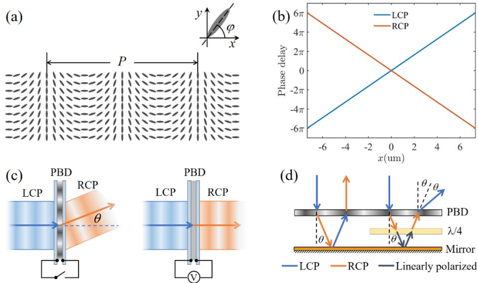
Fig. 7. (a) Top view of the LC director distribution in PBD. (b) Phase delay profile of a PBD with  $15^\circ$  deflect angle at  $\lambda = 633$  nm for LCP and RCP, respectively. (c) Active driving to result in a switching between deflection and non-deflection states. (d) The polarization state change for the LCP wave deflected by PBD and reflected by mirror.
