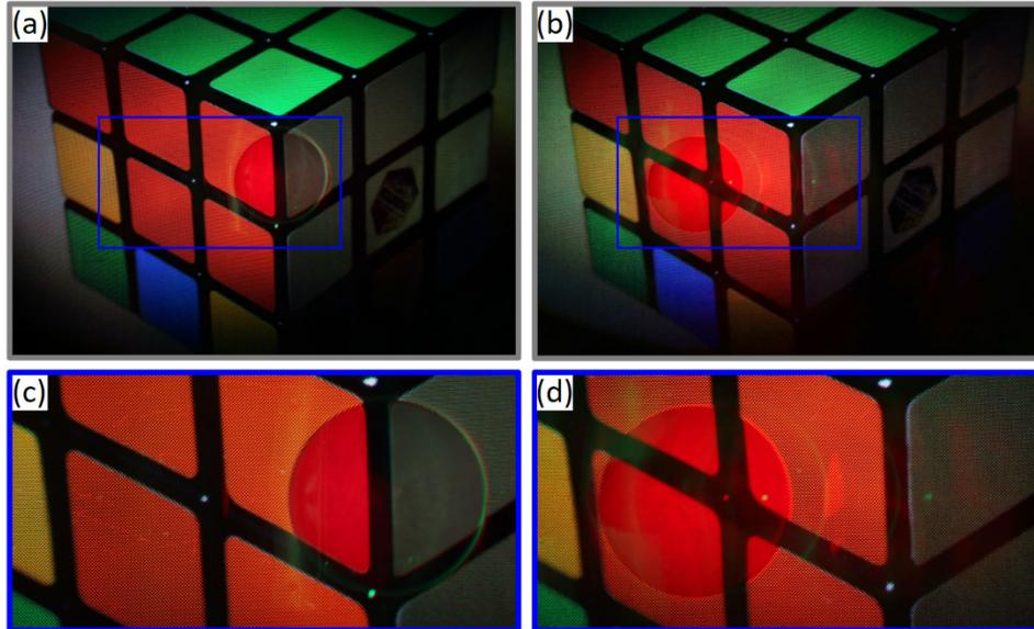
Fig. 8. The experimental results of the proposed multi-resolution display with a PBD as image shifter: a) displayed image with high-resolution region in the center; b) displayed image with shifted high-resolution region; c) the magnified blue rectangle region in (a); d) the magnified blue rectangle region in (b).
