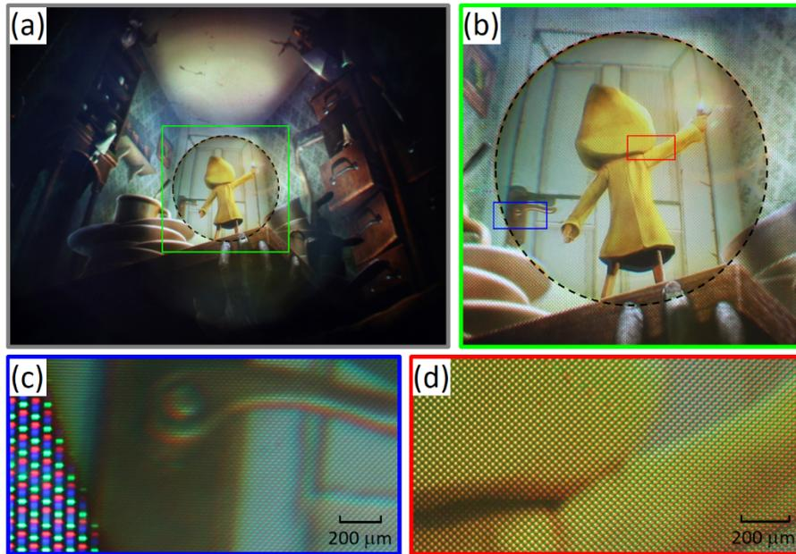
Fig. 4. The experimental photographs with the proposed multi-resolution foveated display with  $4 \times$  resolution enhancement: a) displayed image; b) the magnified green square region in (a); c) the magnified blue rectangle region in (b); d) the magnified red rectangle region in (b).
