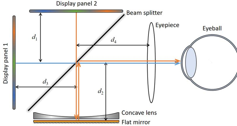
Fig. 2. Schematic diagram of the proposed multi-resolution foveated display for near-eye display devices.
