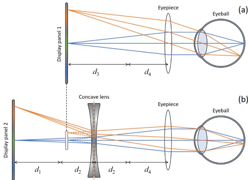
Fig. 3. The unfolded layout of the optical paths for a) display panel 1 and b) panel 2.
