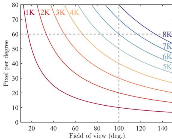
Fig. 1. The trade-off between field of view and angular resolution in near-eye displays for different panel resolutions from 1K to 8K.
