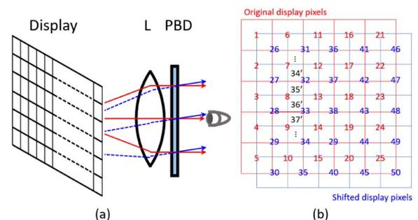
**Fig. 2.** (a) Experimental setup for enhancing resolution with a PBD. (b) Pixel illustration of the original display (sub-frame 1), the shifted display (sub-frame 2), and the combined pixels.
