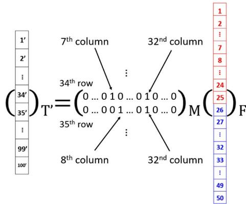
**Fig. 3.** Illustration of the matrix form of adding a low-resolution time-multiplexed display ( $\mathbf{F}$ ) to yield the combined image ( $\mathbf{T}'$ ). The correlation matrix  $\mathbf{M}$  essentially performs an addition operation. For example, the 34th row of  $\mathbf{M}$  adds element #7 and #32 in  $\mathbf{F}$  to yield element #34' in  $\mathbf{T}'$ . Therefore, only the 7th and 32nd elements in the 34th row are 1, and all other are zero.
