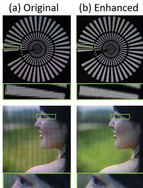
**Fig. 5.** Images captured through a camera for (a) the original resolution and (b) the enhanced resolution for (upper) a “Siemens star” resolution target and (lower) a lady. The green rectangles enclose the magnified regions shown in the pictures. Note that the visible strips are a moiré pattern from the spatial interference of camera and display pixels, and are not visible when directly seen with human eyes.
