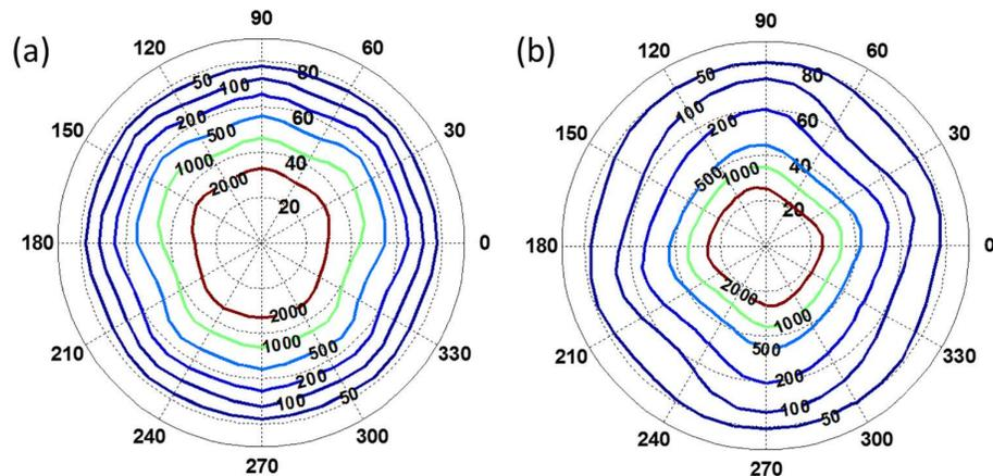
Fig. 11. Simulated ambient isocontrast contour for (a) LCD TV at 50 lux, where  $ACR_{max} = 2931.3:1$ ,  $ACR_{min} = 16.2:1$ , and (b) OLED TV at 50 lux, where  $ACR_{max} = 3362.2:1$ ,  $ACR_{min} = 27.8:1$ . The peak brightness for LCD is 1500 nits and for OLED is 800 nits.
