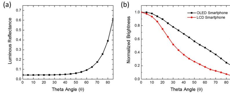
Fig. 8. (a) Calculated luminous reflectance of BK-7 cover glass at different angles, and (b) normalized brightness of LCD and OLED smartphones.
