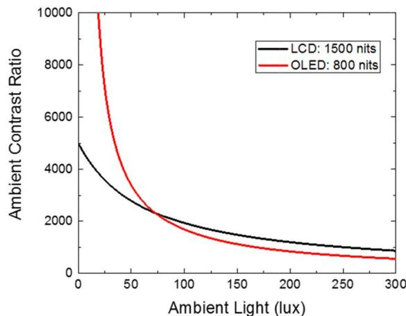
Fig. 4. Calculated ACR as a function of different ambient light conditions for LCD and OLED TVs. Here we assume LCD peak brightness is 1500 nits and OLED peak brightness is 800 nits, and the surface reflectance is 1.5% for both LCD and OLED.
