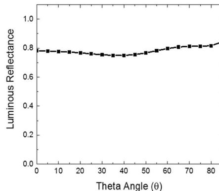
Fig. 7. Calculated angular-dependent luminous reflectance of a multi-layer OLED device.
