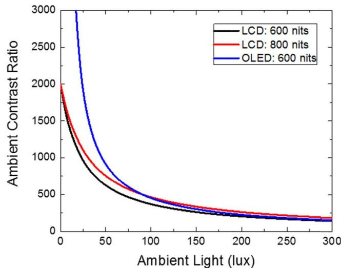
Fig. 3. Calculated ACR as a function of different ambient light conditions for LCD and OLED smartphones. Here, we assume LCD peak brightness is 600/800 nits and OLED peak brightness is 600 nits, and the surface reflectance is 4.2% for both LCD and OLED.
