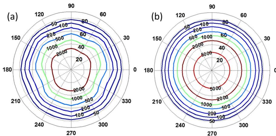
Fig. 13. Simulated ambient isocontrast contour for (a) conventional LCD TV at 50 lux, where  $ACR_{max} = 2931.3:1$ ,  $ACR_{min} = 16.2:1$ , and (b) new LCD TV with mini-LED backlight at 50 lux, where  $ACR_{max} = 7312.5:1$ ,  $ACR_{min} = 18.8:1$ .
