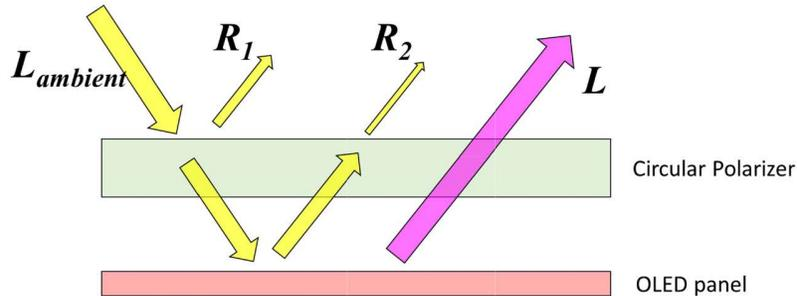
Fig. 2. Schematic diagram of an OLED.
