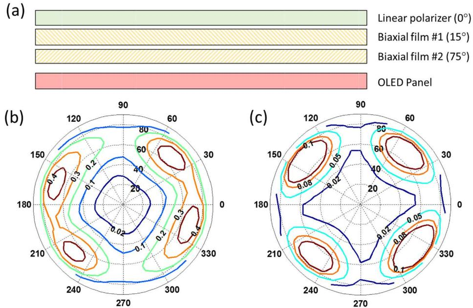
Fig. 14. (a) Schematic diagram of optical configuration of newly proposed broadband and wide-view circular polarizer with two biaxial films; Calculated light leakage for (b) conventional broadband circular polarizer, and (c) new broadband circular polarizer.
