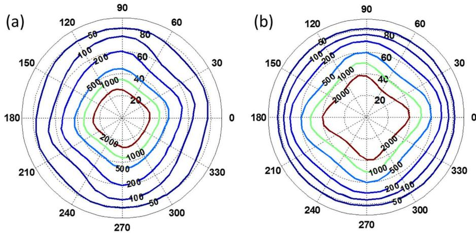
Fig. 15. Simulated ambient isocontrast contour for (a) OLED TV at 50 lux with conventional broadband circular polarizer, where  $ACR_{max} = 3362.2:1$ ,  $ACR_{min} = 27.8:1$ , and (b) OLED TV at 50 lux with new broadband circular polarizer, where  $ACR_{max} = 3363.3:1$ ,  $ACR_{min} = 29.4:1$ .
