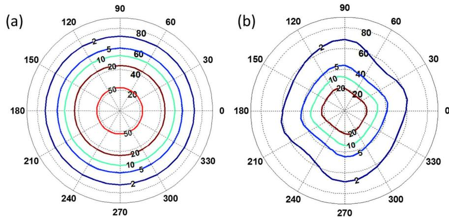
Fig. 12. Simulated ambient isocontrast contour for (a) LCD public display at 10,000 lux, where  $ACR_{max} = 61.2:1$ ,  $ACR_{min} = 1.2:1$ , and (b) OLED public display at 10,000 lux, where  $ACR_{max} = 29.5:1$ ,  $ACR_{min} = 1.2:1$ . The peak brightness for LCD is 2500 nits and for OLED is 1200 nits.
