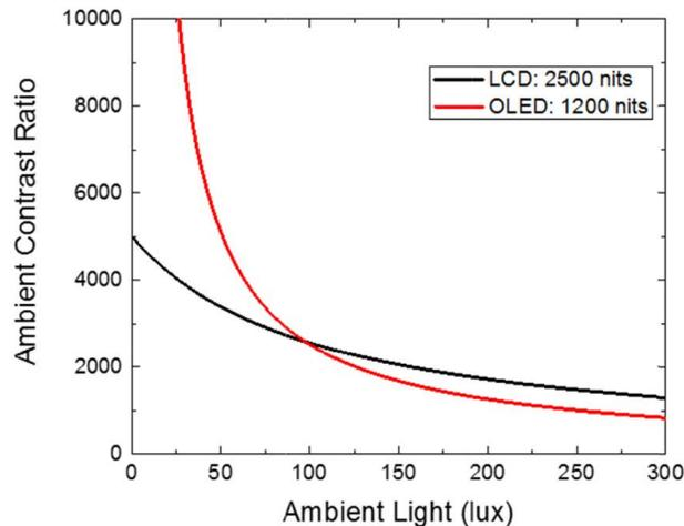
Fig. 5. Calculated ACR as a function of different ambient light conditions for LCD and OLED public displays. Here we assume LCD peak brightness is 2500 nits and OLED peak brightness is 1200 nits, and the surface reflectance is 1.5% for both LCD and OLED.
