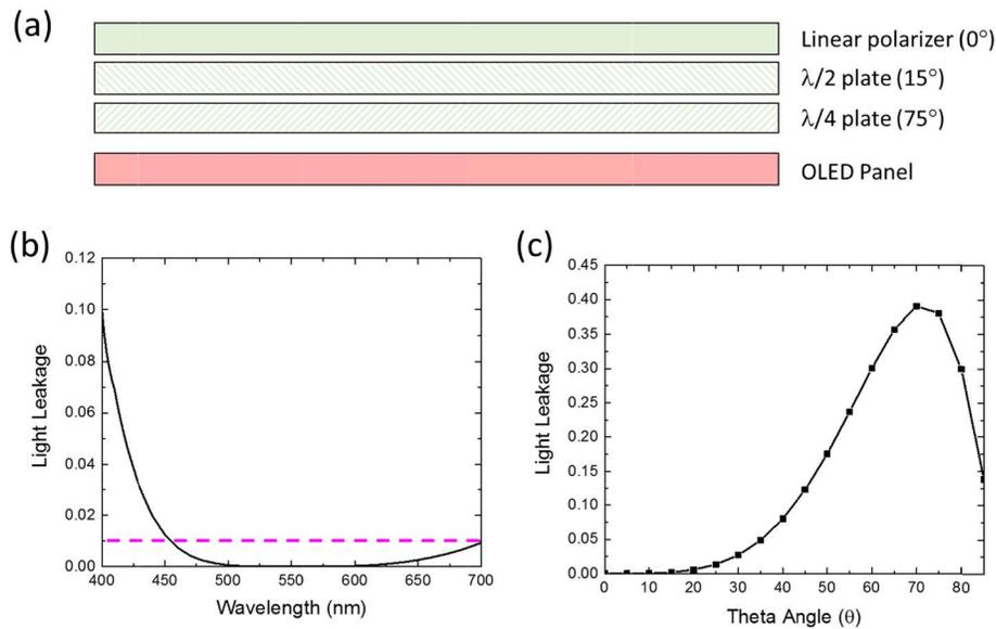
Fig. 6. (a) Schematic diagram of optical configuration of broadband circular polarizer; (b) Calculated light leakage at different wavelengths at normal angle ( $\theta = 0^\circ$ ,  $\varphi = 0^\circ$ ); and (c) Calculated light leakage at different polar angles ( $\varphi = 0^\circ$ ).
