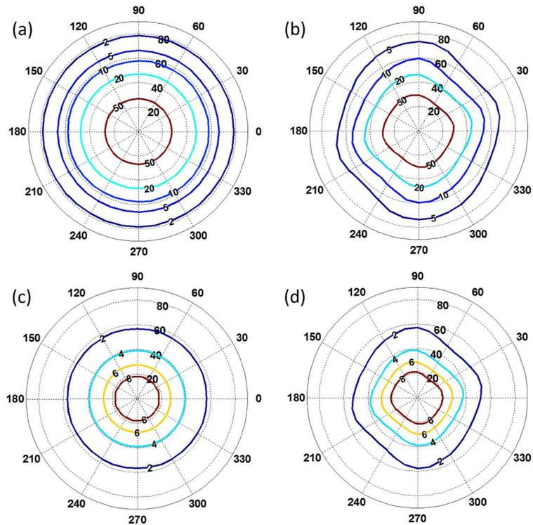
Fig. 9. Simulated ambient isocontrast contour for (a) LCD smartphone at 500 lux, where  $ACR_{max} = 86.1:1$ ,  $ACR_{min} = 1.3:1$ , (b) OLED smartphone at 500 lux, where  $ACR_{max} = 89.2:1$ ,  $ACR_{min} = 2.0:1$ , (c) LCD smartphone at 5000 lux, where  $ACR_{max} = 9.8:1$ ,  $ACR_{min} = 1.1:1$ , and (d) OLED smartphone at 5000 lux, where  $ACR_{max} = 9.8:1$ ,  $ACR_{min} = 1.1:1$ . Both LCD and OLED are assumed to have the same peak brightness: 600 nits.
