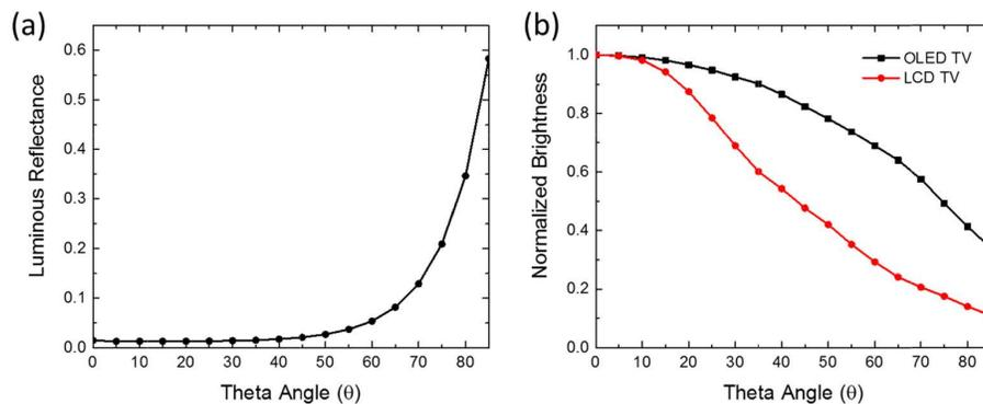
Fig. 10. (a) Calculated luminous reflectance of AR-coated BK-7 cover glass at different angles, and (b) normalized brightness of LCD and OLED TVs.
