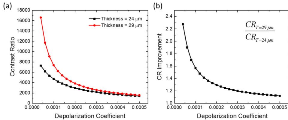
Fig. 8. (a) Simulated contrast ratio and (b) contrast ratio improvement as a function of depolarization coefficient.
