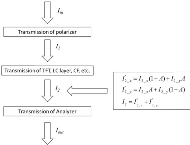
Fig. 3. Flow chart of the proposed simulation model.
