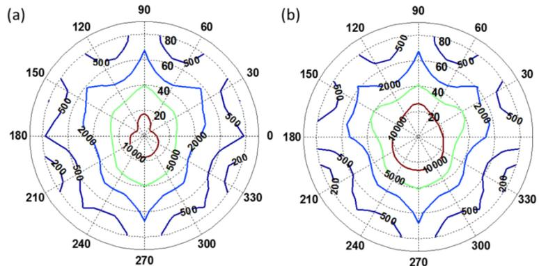
Fig. 15. Simulated isocontrast contour for the proposed device configuration in MVA mode. (a) Polarizer thickness is 24  $\mu\text{m}$ , and (b) polarizer thickness is 29  $\mu\text{m}$ . For the 24- $\mu\text{m}$  thick polarizer:  $CR_{max} = 12,277:1$ ,  $CR_{min} = 132:1$ , and  $CR_{ave} = 4685:1$ . For the 29- $\mu\text{m}$  thick polarizer:  $CR_{max} = 23,163:1$ ,  $CR_{min} = 149:1$ , and  $CR_{ave} = 7223:1$ .
