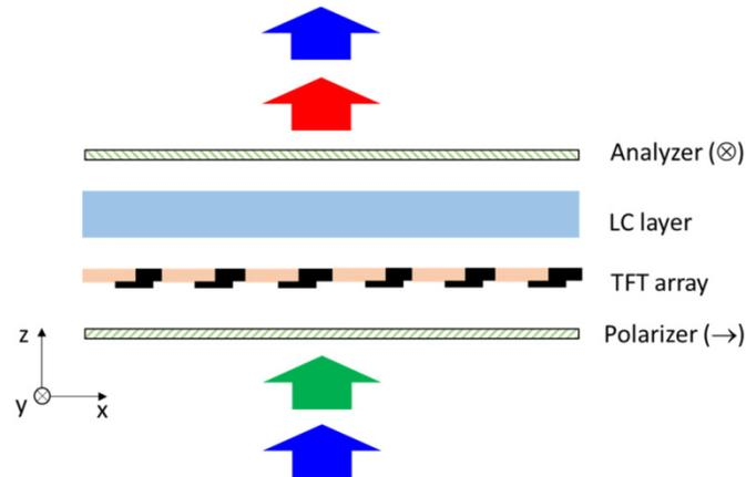
Fig. 19. Schematic diagram of the field-sequential color display.
