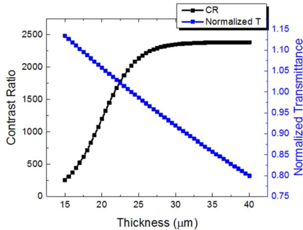
Fig. 7. Simulated contrast ratio and normalized transmittance for FFS mode with depolarization coefficient  $A = 0.00039$ . Note: 24- $\mu\text{m}$  thick polarizer is the reference for  $CR \approx 2000:1$  and efficiency = 1.
