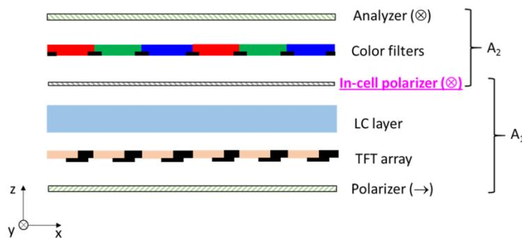
Fig. 12. Schematic diagram of the proposed device structure with an in-cell polarizer.
