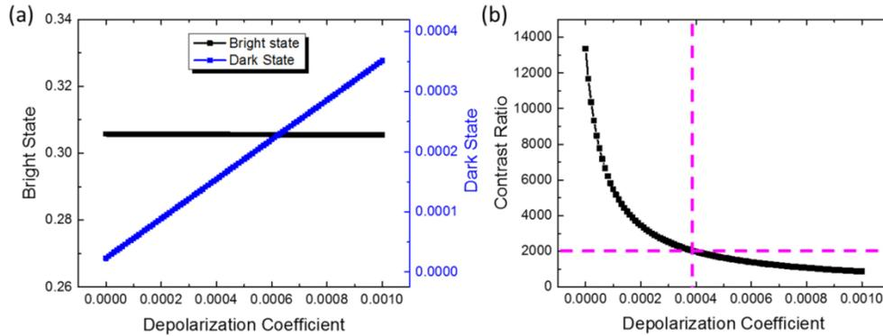
Fig. 6. (a) Simulated transmittance of bright state and dark state, and (b) simulated CR as a function of depolarization coefficient for FFS mode, where depolarization effect is considered.
