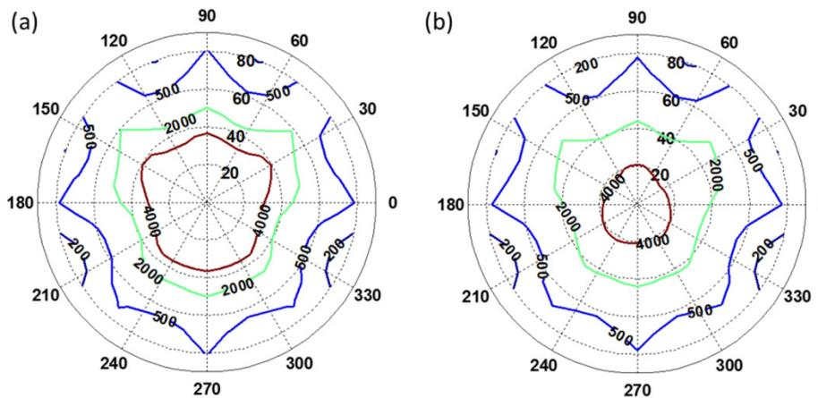
Fig. 9. Simulated isocontrast contour for (a) ideal MVA mode using TechWiz, where  $CR_{max} = 11,437:1$ ,  $CR_{min} = 132:1$ , and  $CR_{ave} = 4350:1$ . (b) Real MVA with  $A=0.00009$ , where  $CR_{max} = 5011:1$ ,  $CR_{min} = 130:1$ , and  $CR_{ave} = 2392:1$ . For both cases, the polarizer thickness is 24 μm.
