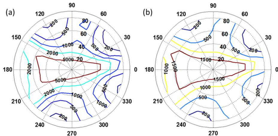
Fig. 11. Simulated isocontrast contour for (a) an ideal FFS mode using TechWiz, where  $CR_{max} = 13,150:1$ ,  $CR_{min} = 105:1$ , and  $CR_{ave} = 4467:1$ . (b) A realistic FFS with depolarization coefficient  $A = 0.00039$ , where  $CR_{max} = 2024:1$ ,  $CR_{min} = 100:1$ , and  $CR_{ave} = 1184:1$ . For both cases, the polarizer thickness is 24  $\mu\text{m}$ .
