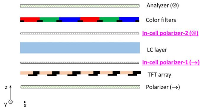
Fig. 17. Schematic diagram of the proposed structure with dual in-cell polarizers. In this case, the polarizer and the analyzer could be removed.
