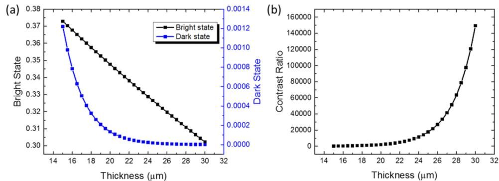
Fig. 1. (a) Simulated transmittance of bright state and dark state, and (b) simulated CR as a function of polarizer thickness. No depolarization effect is considered.
