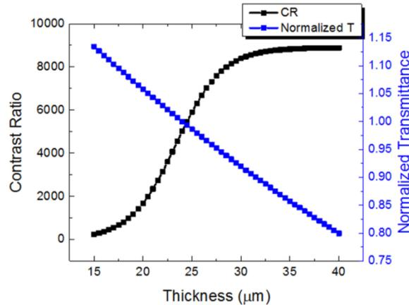
Fig. 5. Simulated contrast ratio and normalized transmittance for MVA mode with depolarization coefficient  $A = 0.00009$ . Note: 24- $\mu\text{m}$  thick polarizer is the reference with CR  $\approx 5000:1$  and efficiency = 1.
