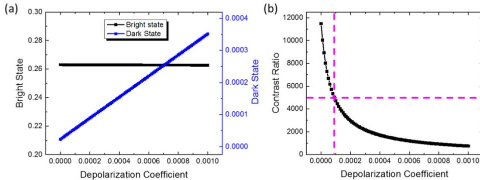
Fig. 4. (a) Simulated transmittance of bright state and dark state, and (b) simulated CR as a function of depolarization coefficient for MVA mode. Depolarization effect is considered.
