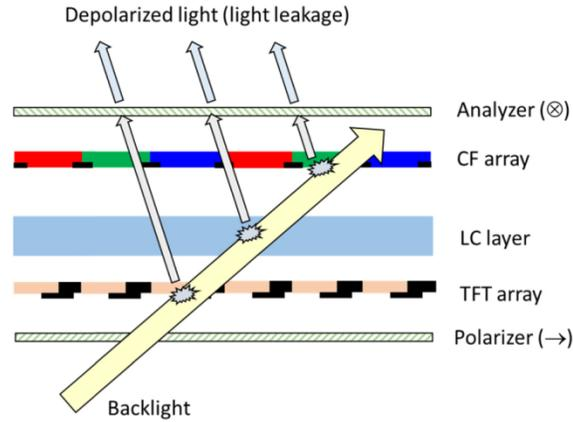
Fig. 2. Schematic diagram for accounting the depolarization effect in an LCD panel. CF: color filter; LC: liquid crystal; TFT: thin-film transistor.
