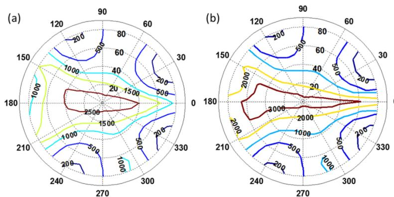
Fig. 16. Simulated isocontrast contour for the new FFS with an in-cell polarizer. (a) Polarizer thickness is 24  $\mu\text{m}$ , and (b) polarizer thickness is 29  $\mu\text{m}$ . For the 24- $\mu\text{m}$  thick polarizer:  $CR_{max} = 3002:1$ ,  $CR_{min} = 115:1$ , and  $CR_{ave} = 1576:1$ . For the 29- $\mu\text{m}$  thick polarizer:  $CR_{max} = 3349:1$ ,  $CR_{min} = 115:1$ , and  $CR_{ave} = 1819:1$ .
