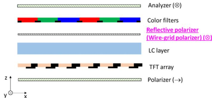
Fig. 18. Schematic diagram of the proposed structure with a reflective polarizer or wire-grid polarizer.
