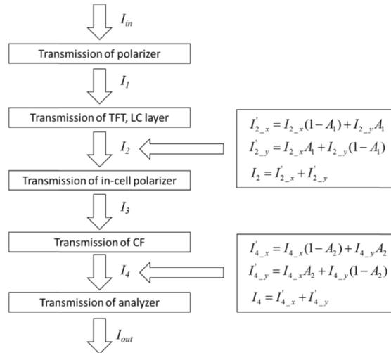
Fig. 14. Flow chart of the proposed simulation model for new structure configuration.
