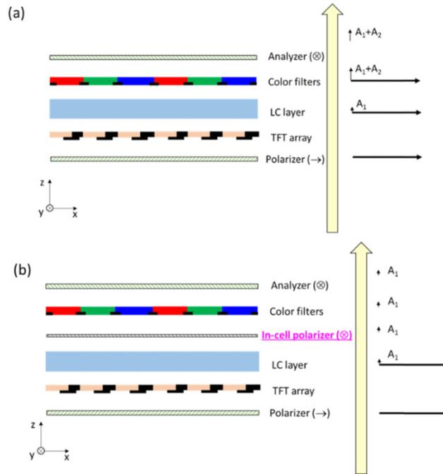
Fig. 13. Working mechanism of (a) conventional LCD panel with depolarization effects, and (b) the proposed LCD panel with decoupled depolarization effects.
