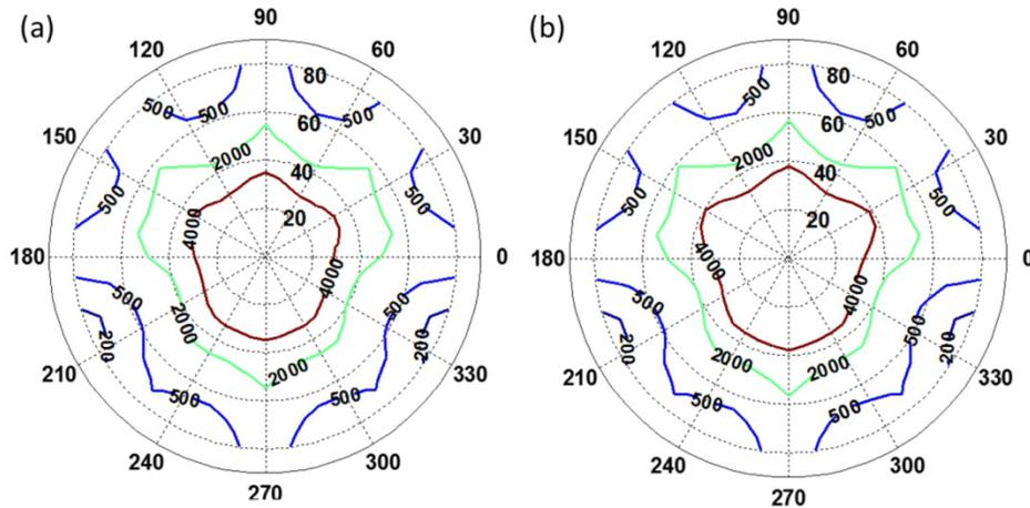
Fig. 10. Simulated isocontrast contour for (a) a realistic MVA with polarizer thickness = 29  $\mu\text{m}$  and  $A = 0.00009$ , where  $CR_{max} = 8129:1$ ,  $CR_{min} = 147:1$ , and  $CR_{ave} = 3501:1$ . (b) Same MVA but with polarizer thickness = 29  $\mu\text{m}$  and  $A = 0.000071$ , where  $CR_{max} = 10,066:1$ ,  $CR_{min} = 148:1$ , and  $CR_{ave} = 4077:1$ .
