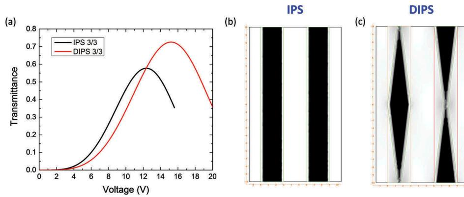
**Figure 3.** (Colour online) (a) Simulated VT curves for conventional protruded IPS and DIPS; brightness profile at on-state voltage for (b) conventional IPS and (c) DIPS ( $w_1 = 3 \mu\text{m}$ ,  $w_2 = 2.5 \mu\text{m}$ ,  $g = 3 \mu\text{m}$ ,  $h = 3.5 \mu\text{m}$  and  $d = 9 \mu\text{m}$  for both IPS and DIPS.  $l = 20 \mu\text{m}$  for DIPS only).
