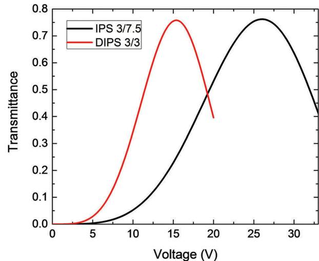
**Figure 7.** (Colour online) Simulated VT curves for conventional IPS and DIPS ( $w_1 = 3 \mu\text{m}$ ,  $w_2 = 2.5 \mu\text{m}$ ,  $g = 7.5 \mu\text{m}$ ,  $h = 3.5 \mu\text{m}$  and  $d = 9 \mu\text{m}$  for IPS;  $w_1 = 3 \mu\text{m}$ ,  $w_2 = 2.5 \mu\text{m}$ ,  $g = 3 \mu\text{m}$ ,  $h = 3.5 \mu\text{m}$ ,  $d = 9 \mu\text{m}$  and  $l = 20 \mu\text{m}$  for DIPS).
