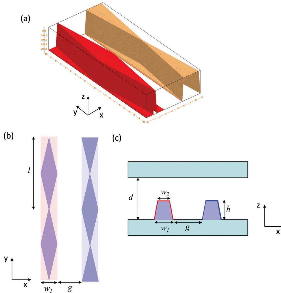
**Figure 1.** (a) Three-dimensional schematic diagram for DIPS; (b) top view and (c) cross-section view for DIPS.
