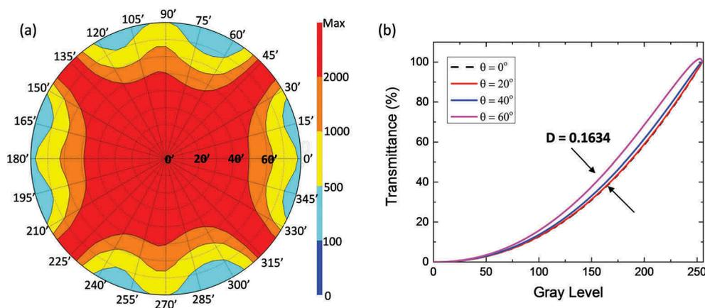
**Figure 8.** (a) Simulated isocontrast contour and (b) viewing angle dependence of gamma curves for biaxial film-compensated two-domain DIPS.
