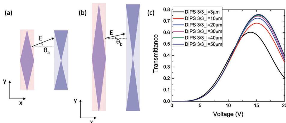
**Figure 5.** (Colour online) Schematic diagram for (a) short diamond electrode and (b) long diamond electrode; (c) simulated VT curves for different diamond lengths ( $w_1 = 3 \mu\text{m}$ ,  $w_2 = 2.5 \mu\text{m}$ ,  $g = 3 \mu\text{m}$ ,  $h = 3.5 \mu\text{m}$  and  $d = 9 \mu\text{m}$ ).
