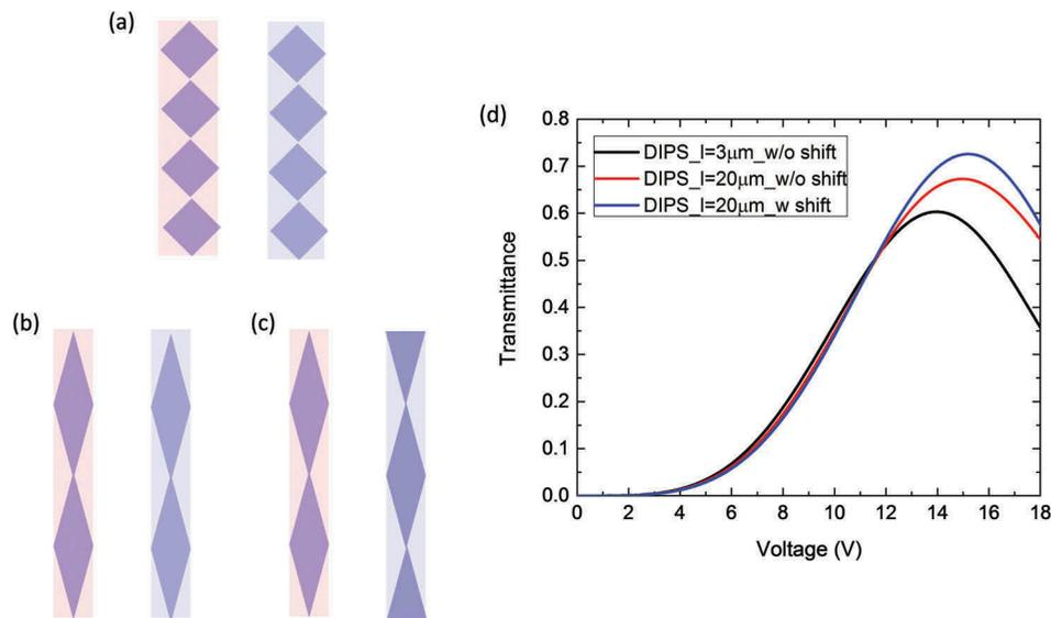
**Figure 6.** (Colour online) Schematic diagram for (a) un-shifted electrode with short diamond, (b) un-shifted electrode with long diamond, (c) shifted electrode with long diamond and (d) simulated VT curves for the structures in (a)–(c) ( $w_1 = 3 \mu\text{m}$ ,  $w_2 = 2.5 \mu\text{m}$ ,  $g = 3 \mu\text{m}$ ,  $h = 3.5 \mu\text{m}$  and  $d = 9 \mu\text{m}$ ).
