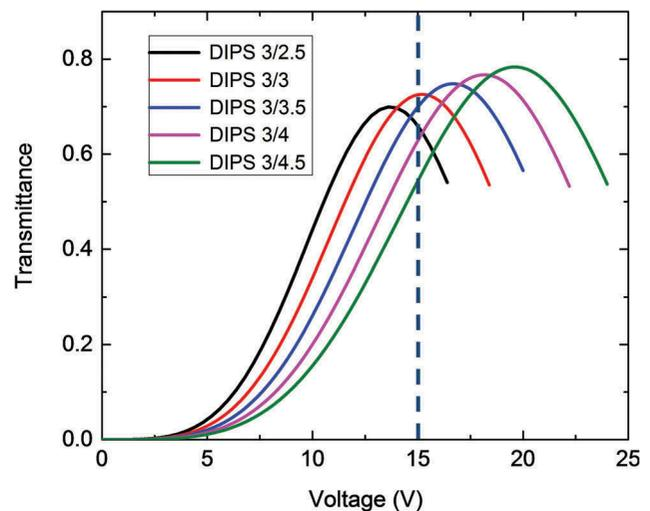
**Figure 4.** (Colour online) Simulated VT curves for different electrode gaps ( $w_1 = 3 \mu\text{m}$ ,  $w_2 = 2.5 \mu\text{m}$ ,  $h = 3.5 \mu\text{m}$ ,  $d = 9 \mu\text{m}$  and  $l = 20 \mu\text{m}$ ).
