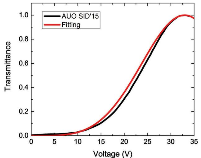
**Figure 2.** Numerical fitting for the VT curve reported in Ref. [16] using extended Kerr model ( $\lambda = 550 \text{ nm}$ ).
