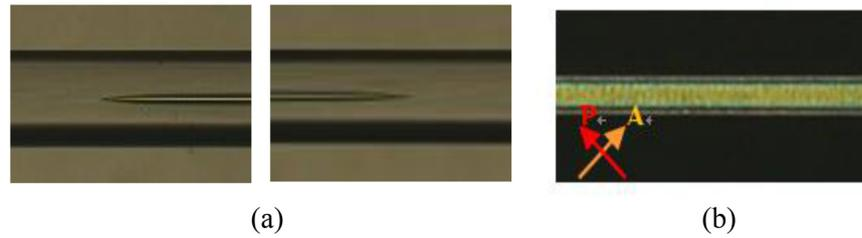
**Figure 3.** Optical microscope image of (a) the tapering structure formed by arc-fusing at both of the spliced ends, and (b) the LC-filled fiber between crossed polarizers.
