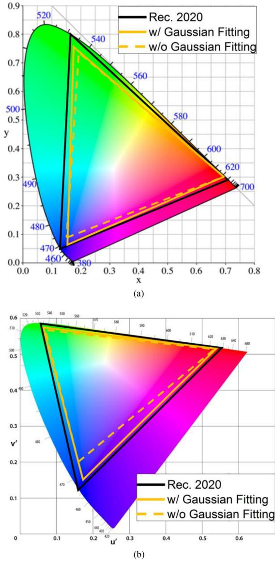
Fig. 10. Simulated color gamut in (a) CIE 1931 and (b) CIE 1976 color space.
