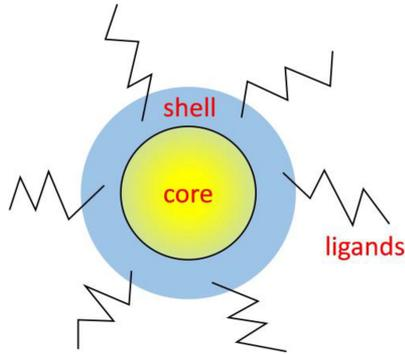
Fig. 1. Schematic diagram of QD's core-shell structure.
