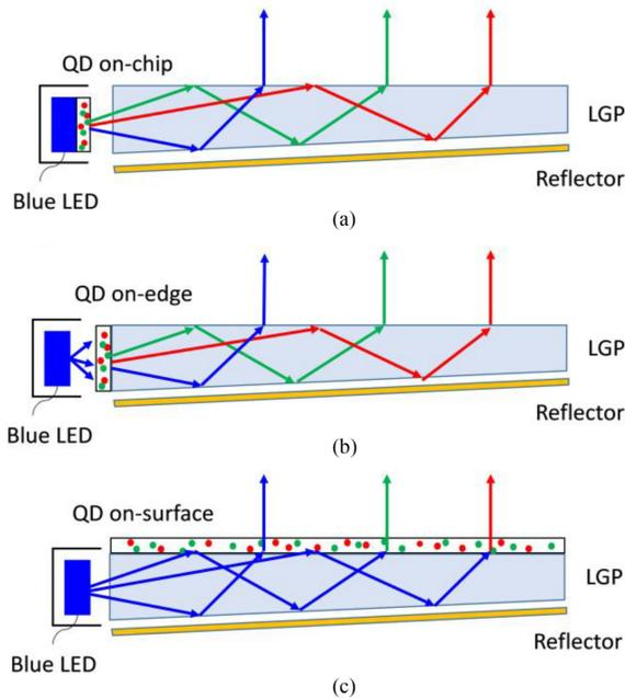
Fig. 3. Schematic diagram for three different device geometries implementing QD mixtures. (a) QD is placed within an LED package. (b) QD is placed between LED and light guide plate, or known as quantum rail. (c) QD is placed on the top surface of light guide plate, or known as quantum dot enhancement film (QDEF). (LGP: light guide plate).
