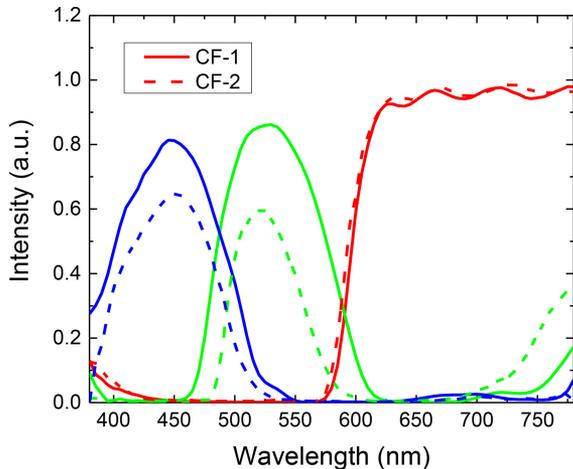
Fig. 11. Transmission spectra of two commercial color filters.
