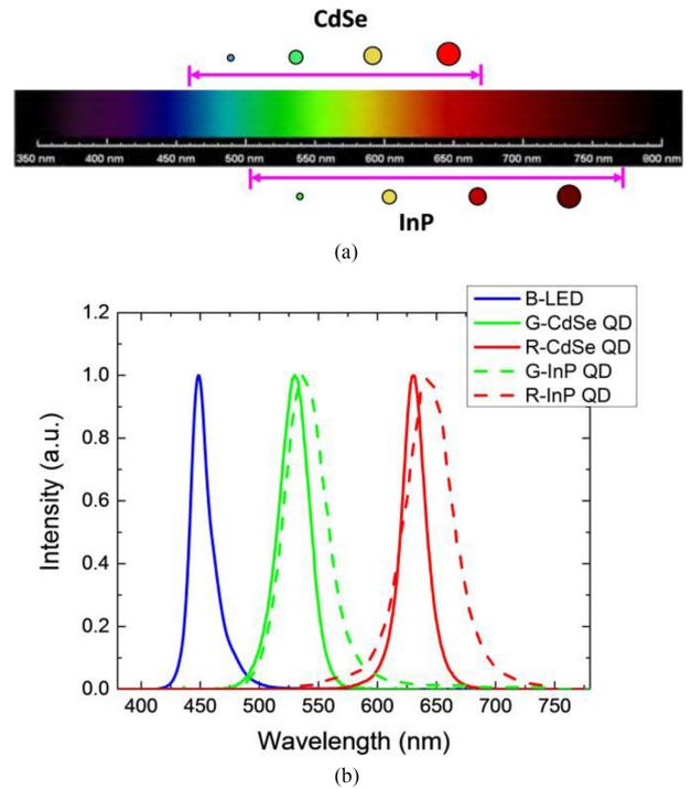
Fig. 2. (a) Potential emission spectral range of CdSe and InP QDs; (b) Typical emission spectra for green and red quantum dots using CdSe (solid line) and InP (dashed line). Blue LED with emission peak  $\lambda = 450$  nm is also shown here.
