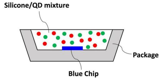
Fig. 4. Schematic diagram of QD on-chip geometry.
