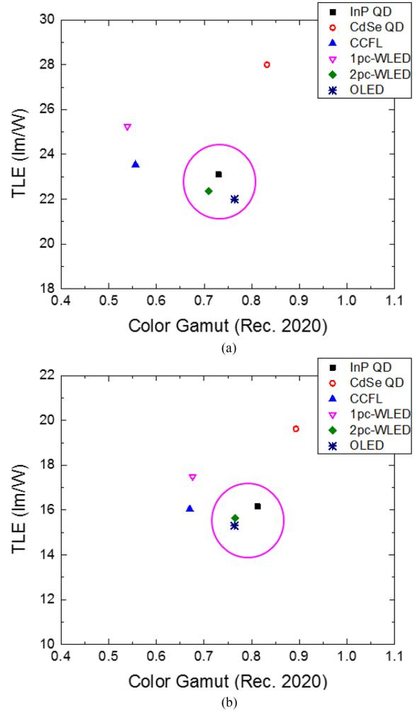
Fig. 12. TLE versus color gamut using (a) CF-1 and (b) CF-2. (Here, color gamut in CIE 1931 color space is employed).
