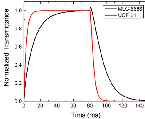
Fig. 6. Simulated response time for UCF-L1 and MLC-6686.
