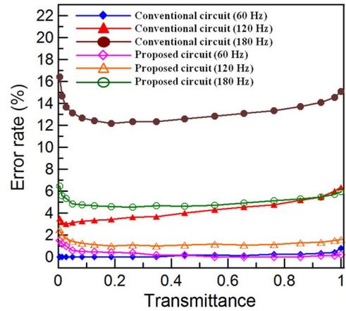
Fig. 5. Simulated stored voltage error rates of conventional circuit and proposed circuit.
