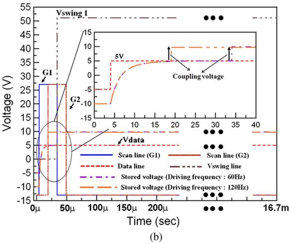
Fig. 3. Stored voltages in  $C_{st}$  with a data voltage. (a) conventional structure and (b) proposed structure.
