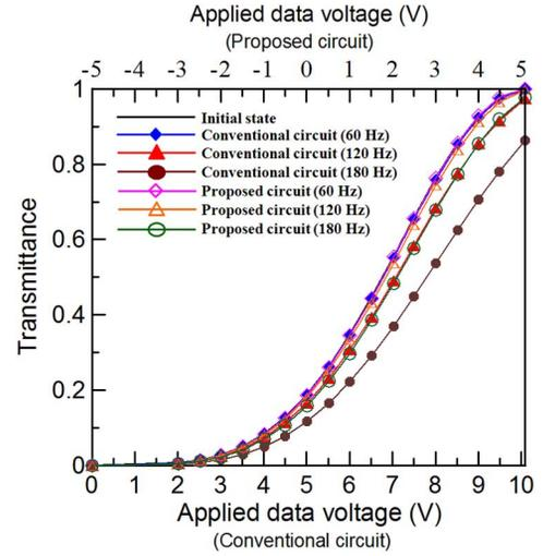
Fig. 4. Simulated VT curves of initial state, conventional circuit, and proposed circuit.
