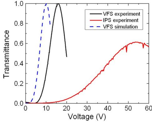
Fig. 1. Measured VT curves for IPS (red) and VFS (black) cells at room temperature ( $T \sim 23^\circ\text{C}$ ). VFS cell: cell gap of  $d = 5.7\ \mu\text{m}$ , incident angle of  $\theta = 70^\circ$  and  $\lambda = 633\ \text{nm}$ . Dashed blue lines represent the simulated curve for a VFS cell with  $d = 3\ \mu\text{m}$ ,  $\theta = 75^\circ$  and  $\lambda = 550\ \text{nm}$
