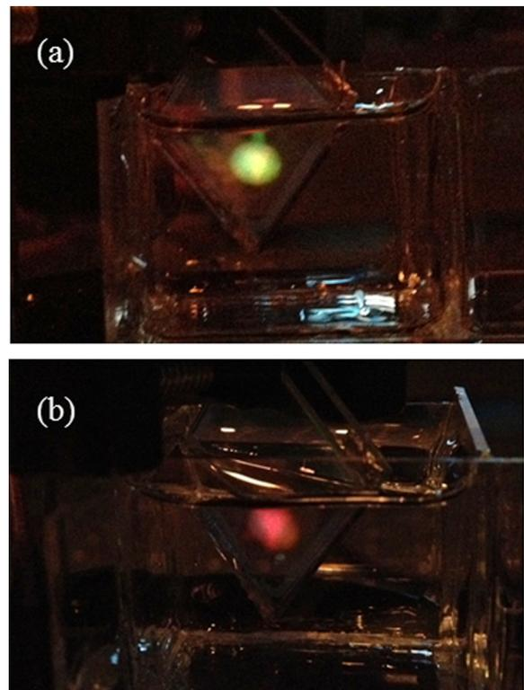
FIG. 6. (a) First order reflection and (b) second order reflection of a BPLC cell. Cell is immersed in water and light is incident at  $\theta \sim 50^\circ$ . Two photos are taken at different angles.
