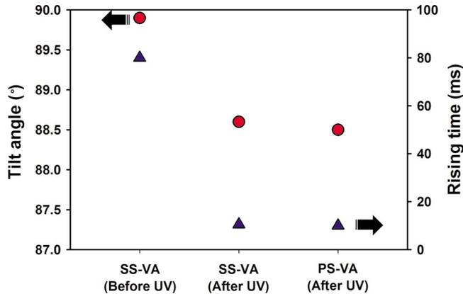
Fig. 2. Tilt angle and rising time of new mode compared with conventional PS-VA mode.
