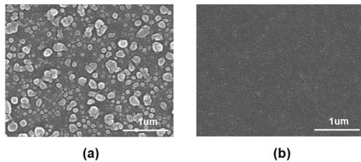
Fig. 3. SEM micrographs of the top surface of alignment layers in: (a) PS-VA and (b) SS-VA modes.
