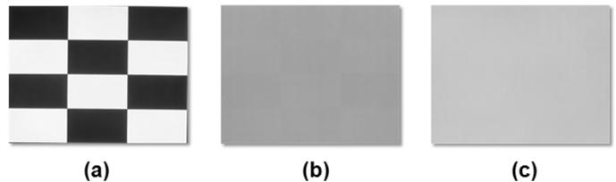
Fig. 5. Photographs of the 46" FHD LCD TV tested at 50 °C for three weeks: (a) image sticking pattern; (b) an image at 100gray/256gray; and (c) an image at 150 gray/256 gray.
