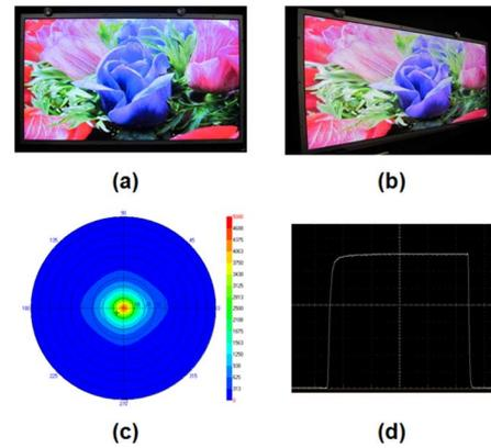
Fig. 4. Photographs and performance of the 46" FHD LCD TV fabricated by SS-VA mode: (a) front view; (b) side view; (c) iso-contrast plot; and (d) measured response time curve of 46" FHD TV.
