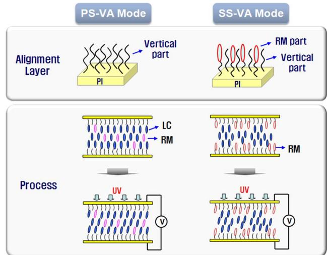
Fig. 1. Schematic diagram of basic concept and manufacturing process of SS-VA mode.
