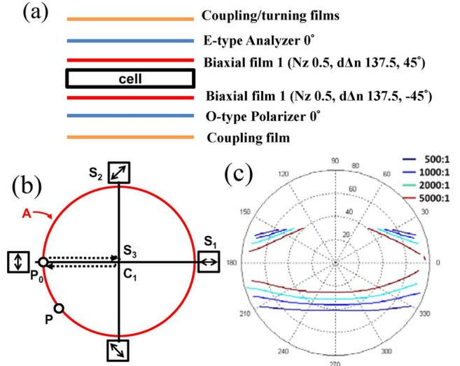
Fig. 11. Proposed VFS BPLCD using an O-type polarizer and an E-type analyzer: (a) film configuration; (b) compensation principle; and (c) simulated isocontrast contours.
