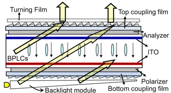
Fig. 1. Device structure of the proposed VFS BPLCD.
