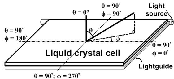
Fig. 2. Polar coordinate of VFS-BPLCD.
