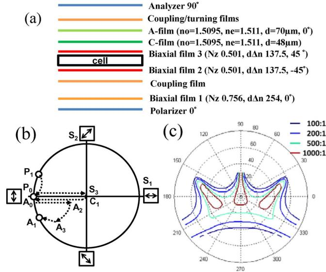
Fig. 7. Biaxial and A/C-films compensated VFS BPLCD: (a) film configuration, (b) compensation principle, and (c) simulated isocontrast contours.
