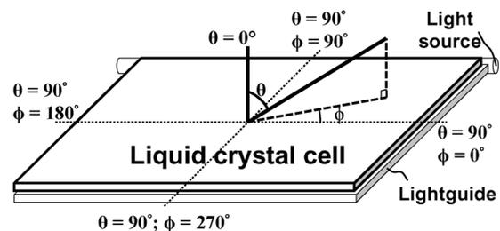
Fig. 2. Polar coordinate of VFS-BPLCD.
