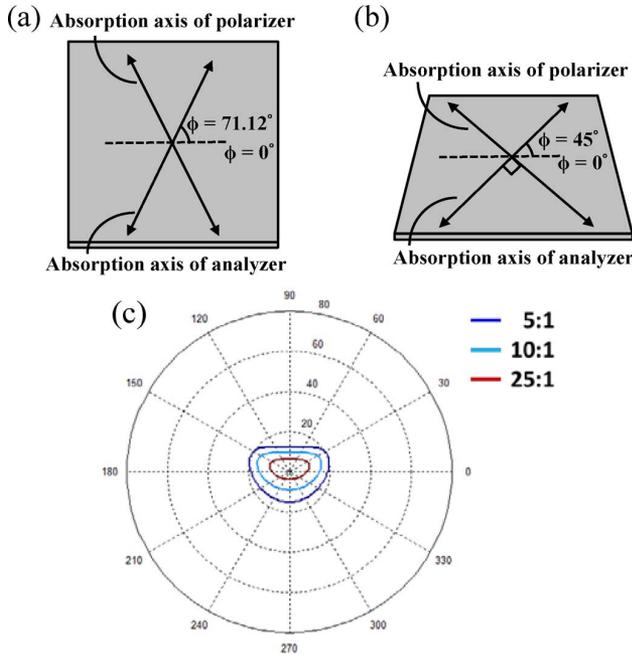
Fig. 3. Change in the effective angle between the polarizer and the analyzer: (a) normal observation ( $\theta = 0^\circ$ ); (b) oblique observation ( $\theta = 70^\circ$ ); and (c) simulated isocontrast contours.
