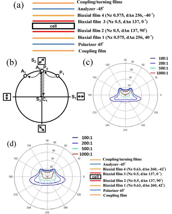
Fig. 6. Optical configuration of a VFS BPLCD with 4 biaxial films: (a) film configuration, (b) compensation principle, and simulated isocontrast contours at  $\theta = 70^\circ$  (c) and  $\theta = 60^\circ$  (d).
