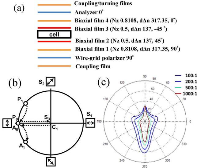
Fig. 9. Optical configuration of the proposed VFS-BPLCD, (a) film configuration, (b) compensation principle, and (c) simulated isocontrast contours.
