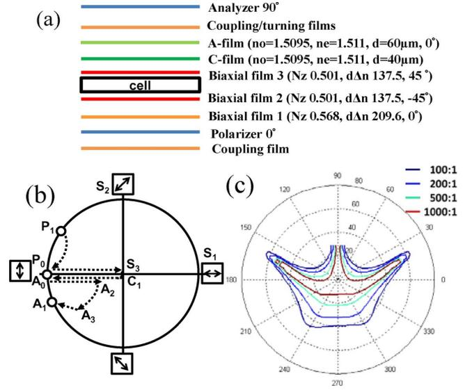
Fig. 8. Film-compensated VFS BPLCD with bottom coupling film laminated to the polarizer: (a) film configuration; (b) compensation principle; and (c) simulated isocontrast contours.
