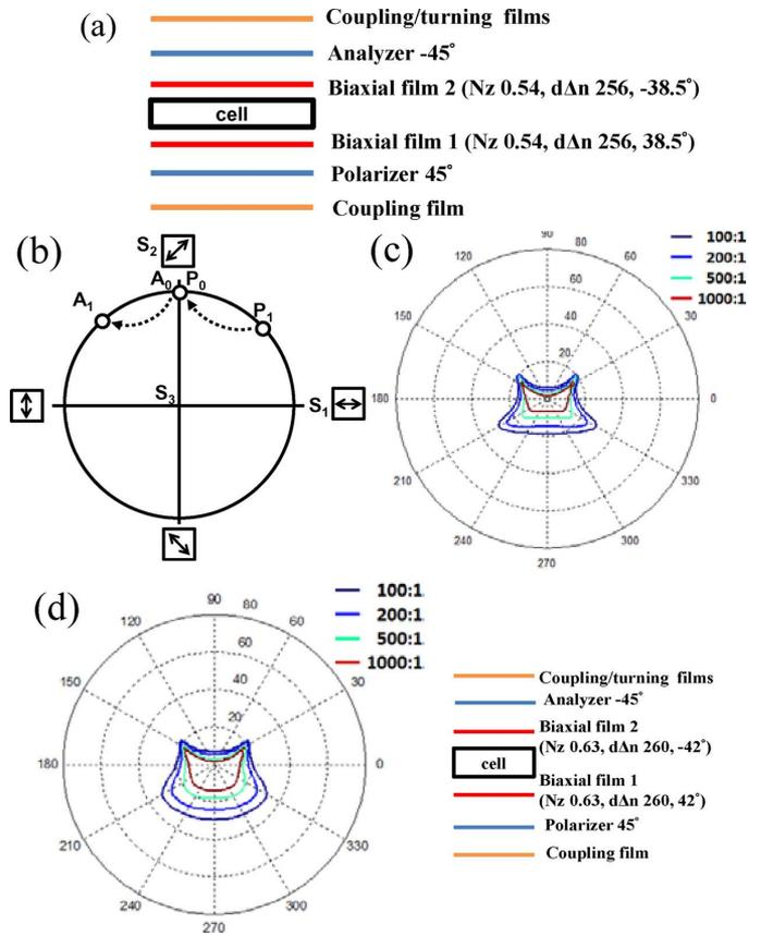
Fig. 4. Biaxial film-compensated VFS BPLCD: (a) device configuration, (b) compensation principle on Poincaré sphere, and simulated isocontrast contours at incident angle  $\theta = 70^\circ$  (c) and  $\theta = 60^\circ$  (d).  $\lambda = 550 \text{ nm}$ .
