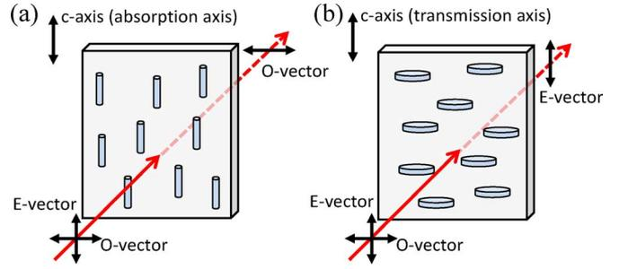
Fig. 10. Schematic drawing of an (a) O-type polarizer and (b) E-type polarizer.
