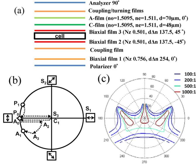
Fig. 7. Biaxial and A/C-films compensated VFS BPLCD: (a) film configuration, (b) compensation principle, and (c) simulated isocontrast contours.
