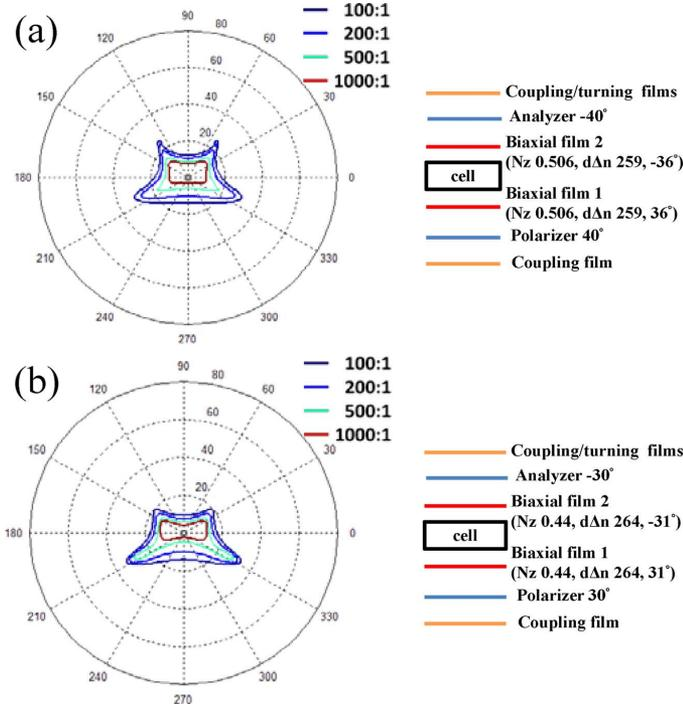
Fig. 5. Simulated isocontrast contours of biaxial film-compensated VFS BPLCD: (a)  $\phi = 40^\circ$  and  $-40^\circ$  and (b)  $\phi = 30^\circ$  and  $-30^\circ$ .
