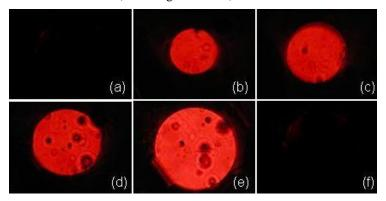
Fig. 3. A droplet cell for red color light switch at voltages of (a) V=0, (b) V=60, (c) 38, (d) 33, and (e) V=22 Volts. (f) (Media 2) Shows the dynamic response of the red droplet with a pulsed voltage (55 Volts) applied to the cell. The red droplet aperture ~260  $\mu$ m and cell gap ~200  $\mu$ m.
