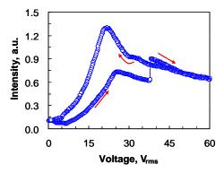
Fig. 4. Measured voltage dependent light transmittance. The red arrow indicates voltage increasing or decreasing direction. The aperture of the red droplet is ~260 µm and the cell gap is ~200 µm.
