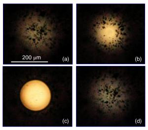
Fig. 2. A droplet cell for proving the proposed operation mechanism at (a) V = 0, (b) V = 25 Volts, and (c) V = 40 Volts. (d) (Media 1) The dynamic response of the droplet with a pulsed voltage (40 Volts) applied to the cell. The droplet aperture is ~340  $\mu$ m and cell gap is ~200  $\mu$ m.
