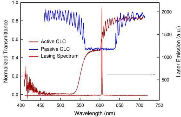
Fig. 3. The normalized transmittance of active CLC (brown line) and passive CLC (blue line). The red line shows the lasing spectrum of the active CLC cell at 10  $\mu\text{J}/\text{pulse}$  pump.
