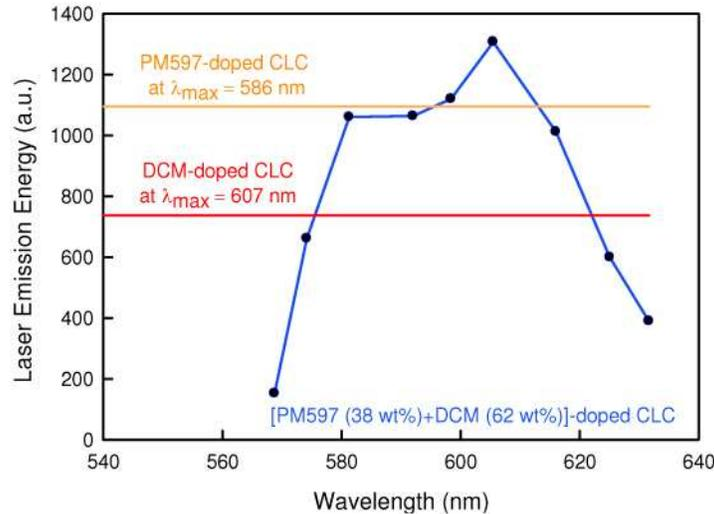
Fig. 1. The laser emission energy of binary-dye doped CLC vs. wavelength (blue line), PM597-CLC at  $\lambda = 586$  nm (orange line), and DCM-CLC at  $\lambda = 607$  nm (red line). Pump energy = 25  $\mu$ J/pulse for all the measurements.
