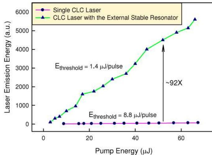
Fig. 4. The laser emission energy dependence on the pump energy of a single CLC laser (pink line) and a CLC laser with an external stable resonator (green line). In this experiment, because the laser output with an external stable resonator is significantly higher than that of the single CLC laser, in order to show this contrast an arbitrary scale which is different from Fig. 1 is used.
