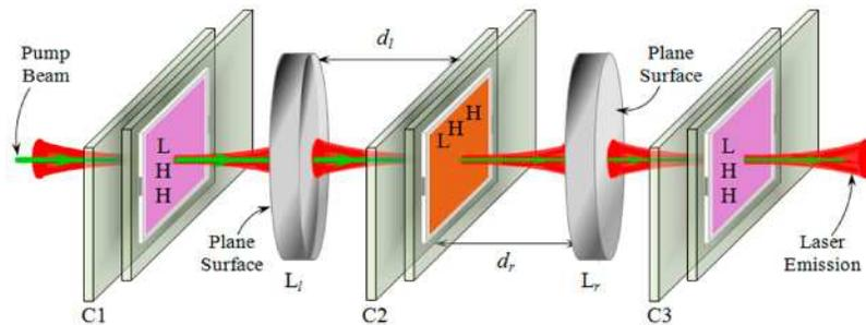
Fig. 2. A schematic diagram of the CLC laser including an external stable resonator. C1 and C3: CLC reflectors;  $L_l$  and  $L_r$ : plano-convex lenses; C2: the active CLC cell. C1 and C3 are, in practice, fixed on the plane surfaces of  $L_l$  and  $L_r$ , respectively.
