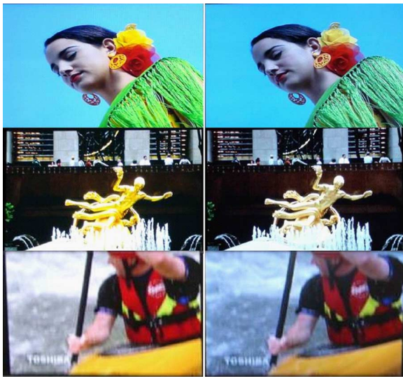
Fig. 6. Photos from a 32" MVA LCD TV prototype. Left column: five-primary (RGBYC); right column: conventional RGB primaries. Backlight: CCFL in both systems.
