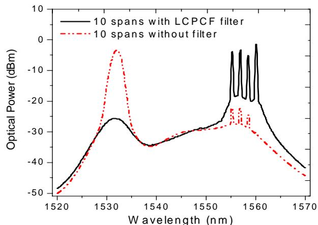
Fig. 1. Optical power spectrum after 10 spans with and without the LCPCF filter. Without filtering, a large ASE peak is created at 1530 nm and the signals drown in noise.
