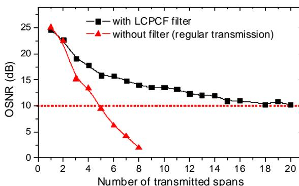
Fig. 5. Results of OSNR vs. number-of-spans investigation without filtering and with the LCPCF filter. Each span here is of fixed length 80 km.
