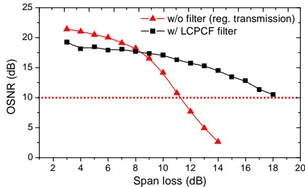
Fig. 4. Results of OSNR vs. span-loss investigation without filtering and with the LCPCF filter. The number of transmitted spans was fixed at 10.
