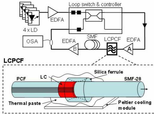
Fig. 3. Experimental loop setup used to demonstrate LCPCF noise filtering. The bottom enlargement illustrates the physical layout of the LCPCF filter.
