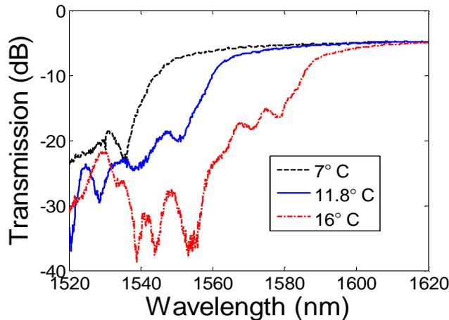
Fig. 2. Transfer curve (filter shape) of the LCPCF filter for three different temperatures. The length of the PCF is 50 cm and the LC infiltrated region is 10 mm.
