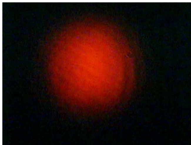
FIGURE 3 Probing beam image of the He-Ne laser snap shot by CCD, 150 s after the sample was cured by CPC with a total of 20 laser pulses
