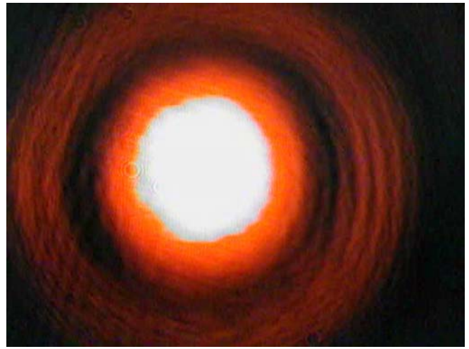
FIGURE 5 Probing beam image of the He-Ne laser snap shot by CCD 150 s after the fourth grouped pulses exposure on the sample film
