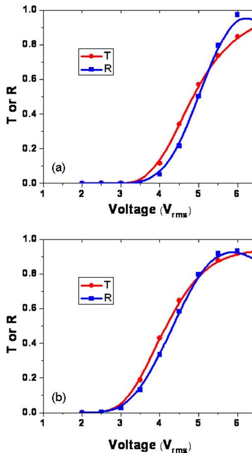
FIG. 5. (Color online) Voltage-dependent reflectance and transmittance curves for (a)  $W=2 \mu\text{m}$ ,  $G=5 \mu\text{m}$ ,  $V_{\text{bias}}=0 V_{\text{rms}}$ , and rubbing angle  $\phi=90^\circ$  and (b)  $W=3 \mu\text{m}$ ,  $G=6 \mu\text{m}$ ,  $V_{\text{bias}}=1.5 V_{\text{rms}}$ , and rubbing angle  $\phi=50^\circ$ .
