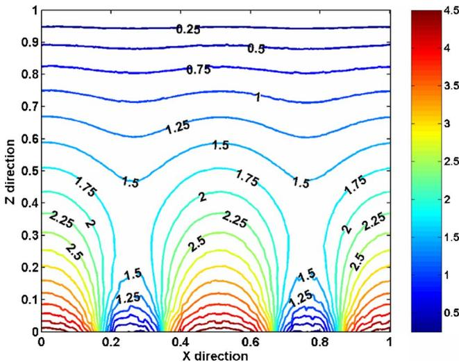
FIG. 2. (Color online) Equal-potential lines in the LC cell region for one sample section with  $6 V_{\text{rms}}$  applied to pixel electrode and the reflectors are commonly biased at  $0 V_{\text{rms}}$ .
