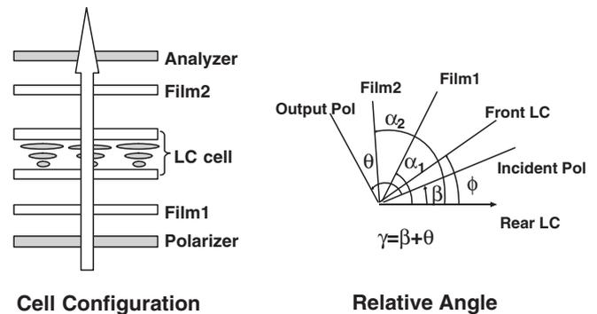
Fig. 1. Device configuration and orientation angles of the linear polarization converter.
