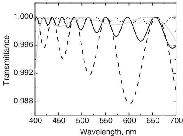
Fig. 4. Normalized transmission spectrum of a single  $90^\circ$  TN LC cell with different cell gap between crossed polarizers. Black dashed line:  $d\Delta n = 5\lambda$ , black solid line:  $d\Delta n = 10\lambda$ , black dot line:  $d\Delta n = 20\lambda$ , and grey solid line: the present design.
