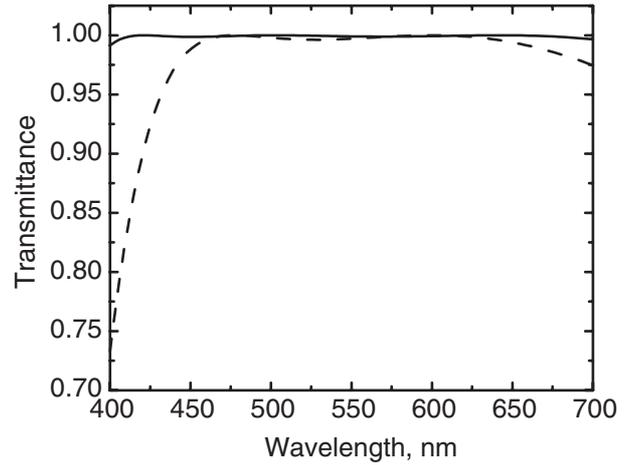
Fig. 5. Normalized transmission spectrum for a device obtained by the Jones method (solid line) and by the Poincaré Sphere method (dashed line).
