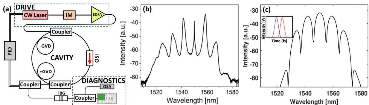
Fig. 2. (a) Experimental schematic, (b) experimental broadband output optical spectrum, and (c) simulated spectral interference pattern corresponding to the closely separated stretched-pulse soliton temporal intensity profile inset.
