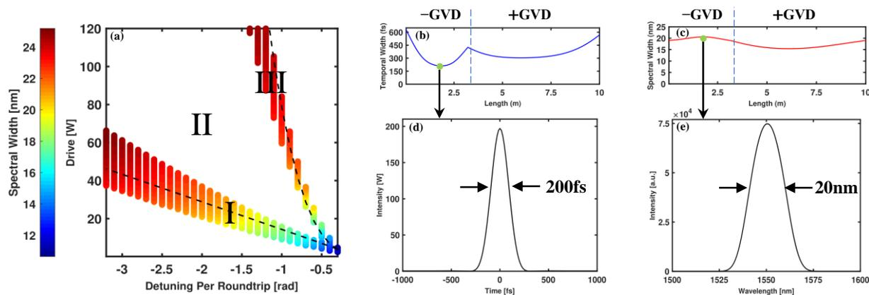
Fig. 1. (a) Stable solutions from numerical simulations with varying drive power and detuning for a fiber cavity with a total length of 10 m and net GVD of  $-8000 \text{ fs}^2$ . Important regions are indicated with Roman numerals. (b) Temporal and (c) spectral width evolution in the cavity with drive power of 15 W and detuning of  $-1.5 \text{ rad}$ , and (d) temporal and (e) spectral intensity profile of the shortest pulse in the cavity.
