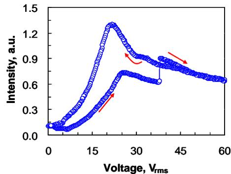
Fig. 4. Measured voltage dependent light transmittance. The red arrow indicates voltage increasing or decreasing direction. The aperture of the red droplet is  $\sim 260 \mu\text{m}$  and the cell gap is  $\sim 200 \mu\text{m}$ .
