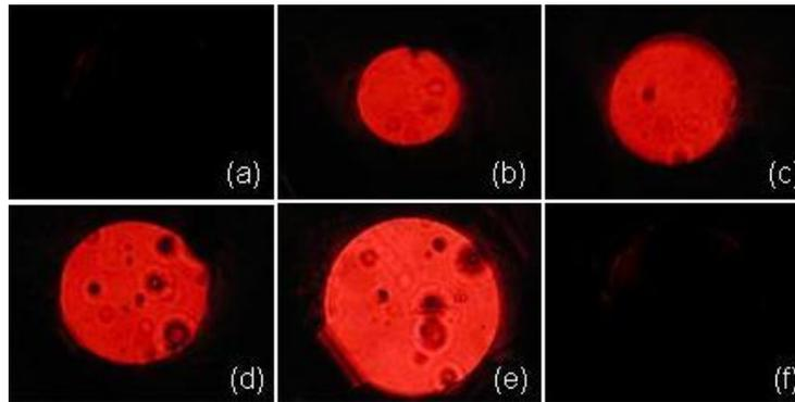
Fig. 3. A droplet cell for red color light switch at voltages of (a)  $V = 0$ , (b)  $V = 60$ , (c) 38, (d) 33, and (e)  $V = 22$  Volts. (f) (Media 2) Shows the dynamic response of the red droplet with a pulsed voltage (55 Volts) applied to the cell. The red droplet aperture  $\sim 260 \mu\text{m}$  and cell gap  $\sim 200 \mu\text{m}$ .
