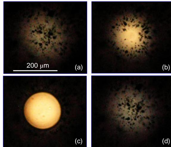
Fig. 2. A droplet cell for proving the proposed operation mechanism at (a)  $V = 0$ , (b)  $V = 25$  Volts, and (c)  $V = 40$  Volts. (d) (Media 1) The dynamic response of the droplet with a pulsed voltage (40 Volts) applied to the cell. The droplet aperture is  $\sim 340$   $\mu\text{m}$  and cell gap is  $\sim 200$   $\mu\text{m}$ .
