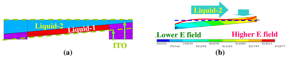
Fig. 2. (a) Device geometry for the electric field simulation. (b) Simulated electric field distribution of liquid-1 and shape of the interface between two liquids in a voltage-on state. The blue dashed lines represent the ideal shape of the interface and the red solid line represents the actual shape of the interface.
