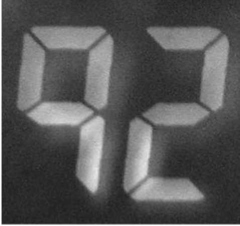
Figure 3. The displayed image using a dye-doped T-PDLC reflective display at V=20 \text{ V}_{\text{rms}} . White paper was placed behind the bottom substrate as a diffusive reflector. Black dye concentration: 2%, LC/polymer mixture: NOA65: E48=40:60, d=6.7 \mu\text{m} (11).
