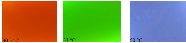
Fig. 5: Temperature dependent CLC bandpass filters.
