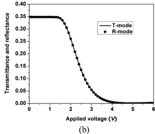
Fig. 12. Dual-cell-gap transfective ECB LCDs (a) schematic device configuration and (b) voltage dependent transmittance and reflectance curves.
