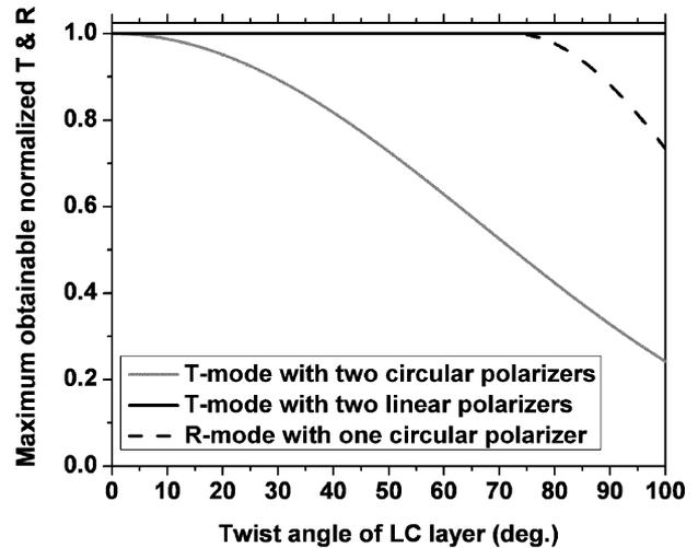
Fig. 9. Maximum obtainable normalized reflectance and transmittance in the transfective MTN LCD and the transfective TN LCD as a function of twist angle.
