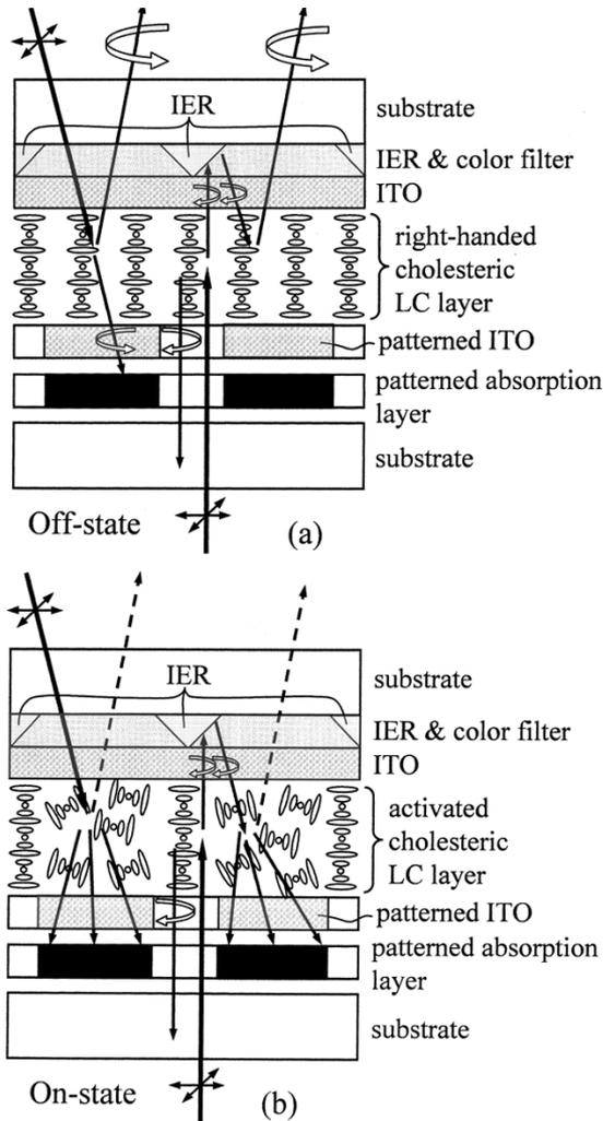
Fig. 5. Schematic configuration of reflection type transfective cholesteric LCD and its operating principles at (a) off-state and (b) on-state.
