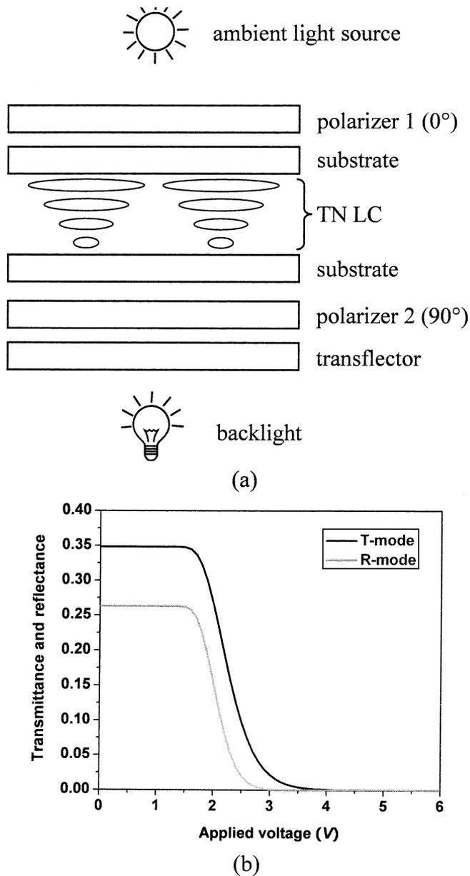
Fig. 6. Transflective TN LCDs. (a) Schematic device configuration. (b) Voltage dependent transmittance and reflectance curves.
