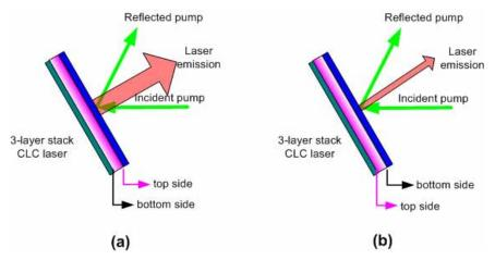
Fig. 4. Sample layout in the experimental setup: (a) top side of the active film is facing the pump beam and (b) bottom side of the active film is facing the pump beam. The 3-layer stack CLC laser: mirror (dark green) / active CLC film (magenta) / passive CLC film (blue).
