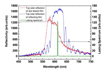
Fig. 2. Top side reflection bands of the 15  $\mu$ m active film (red) and the 8  $\mu$ m passive film (blue), and the lasing spectrum at 53  $\mu$ J/pulse pump (green).
