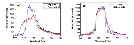
Fig. 6. The top side (blue) and bottom side (red) reflection bands of the CLC polymer film: (a) the 15  $\mu$ m dye-doped CLC polymer film (b) the 8  $\mu$ m passive CLC polymer film.
