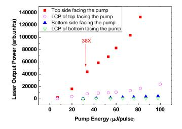
Fig. 5. The pump energy dependent laser output power from a single 15  $\mu m$  active CLC film with the top side facing the pump source and the bottom side facing the pump source.
