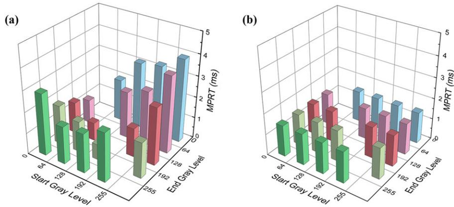
**FIGURE 10** — (a) The gray-to-gray response time of the hole-type vertical alignment–fringe-field switching mode. (b) Motion picture response time (MPRT) at  $f = 90$  Hz with duty ratio = 0.17,  $T_g = 5$  ms.
