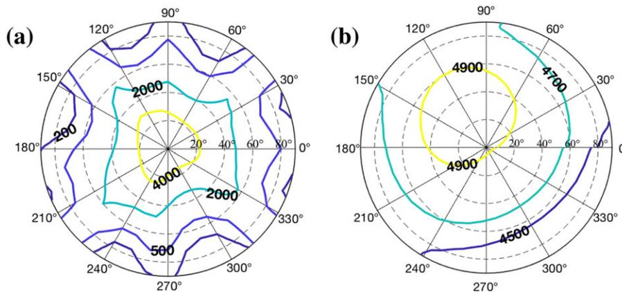
**FIGURE 8** — Simulated isocontrast contours (a) with conventional backlight and (b) with directional backlight and compensation films. The full width at half maximum of the directional backlight is 20° (+10°/−10°).
