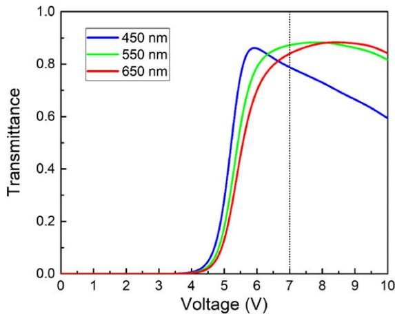
**FIGURE 7** — Simulated voltage-transmittance curves of the proposed vertical alignment-fringe-field switching cell at the specified wavelengths;  $d = 3.5 \mu\text{m}$ ,  $w = 4 \mu\text{m}$ , and  $g = 3 \mu\text{m}$ .
