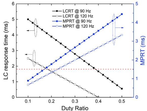
**FIGURE 3** — The motion picture response time (MPRT, blue) and liquid crystal response time (LCRT, black) as a function of duty ratio with  $T_g = 5$  ms. The red dashed lines represent MPRT = 1.5 ms.
