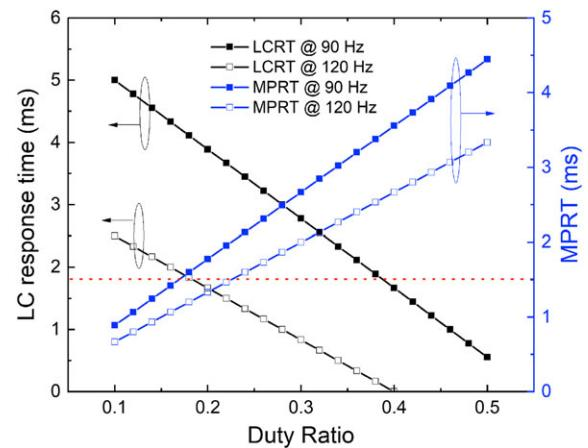
FIGURE 3 — The motion picture response time (MPRT, blue) and liquid crystal response time (LCRT, black) as a function of duty ratio with  $T_g = 5$  ms. The red dashed lines represent  $MPRT = 1.5$  ms.
