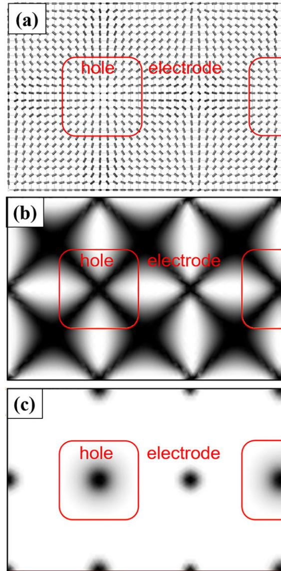
**FIGURE 6** — Top view of (a) simulated liquid crystal director distributions and on-state transmittance profiles of the vertical alignment-fringe-field switching cell with crossed (b) linear polarizers and (c) circular polarizers, at  $V_{\text{On}} = 7 \text{ V}_{\text{rms}}$ .
