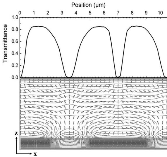
**FIGURE 5** — Transmittance (upper) and cross-sectional view of simulated liquid crystal director distributions (lower) of the vertical alignment-fringe-field switching cell at  $7 \text{ V}_{\text{rms}}$ .
