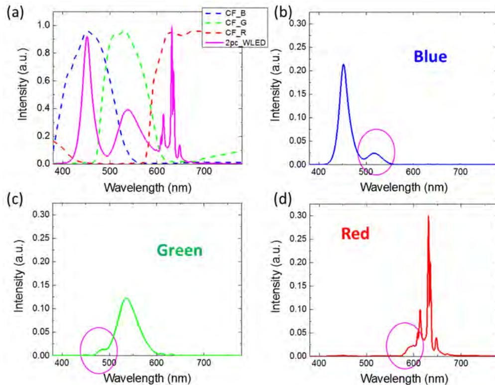
Fig. 1. (a) Transmission spectrum for commercial color filters and 2pc-WLED with green ( $\beta$ -sialon:Eu<sup>2+</sup>) and red ( $K_2SiF_6:Mn^{4+}$ ) phosphors; (b)-(d) Output spectrum for the blue, green and red sub-pixels, respectively.
