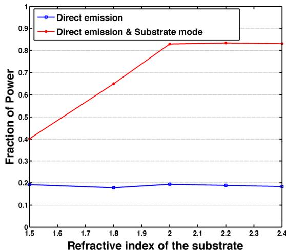
**Figure 2.** How the refractive index of the substrate influence the light outcoupling of the red QLED
