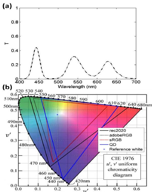
**Figure 5.** (a) Emission spectra of the RGB QLED display and (b) the color gamut of the RGB QLED display.
