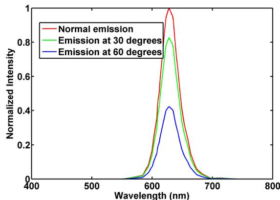
**Figure 3.** Emission spectra of the red QLED under different angles
