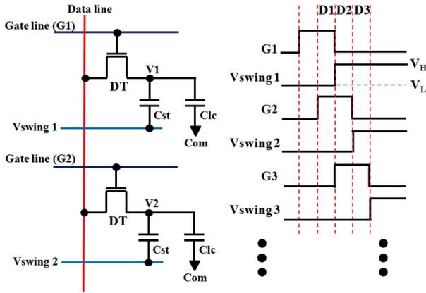
Fig. 2. Proposed driving scheme and its timing diagram.
