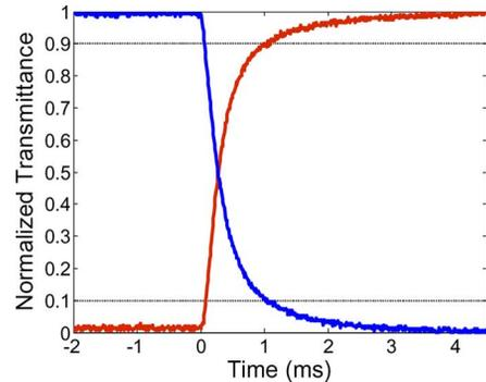
Fig. 4. Measured rise time and fall time of the VFS-BPLC cell.  $\theta_i = 45^\circ$ ,  $\lambda = 633 \text{ nm}$ , and  $T \sim 23 \text{ }^\circ\text{C}$ .
