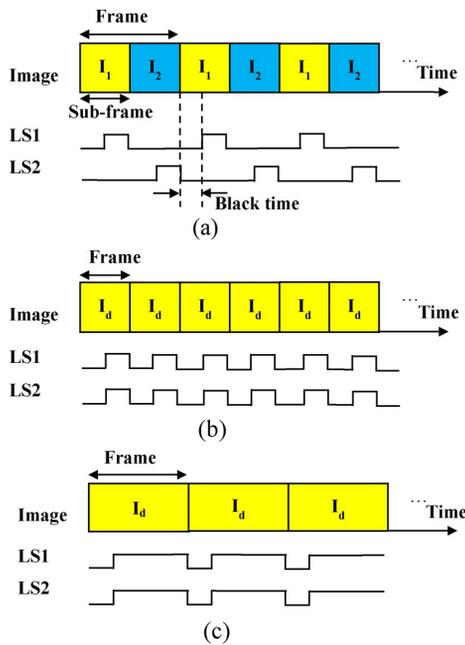
Fig. 6. Driving schemes of the proposed display device: (a) dual-view mode at refresh rate of 120 Hz; (b) identical-view mode at refresh rate of 120 Hz; and (c) identical-view mode at refresh rate of 60 Hz.
