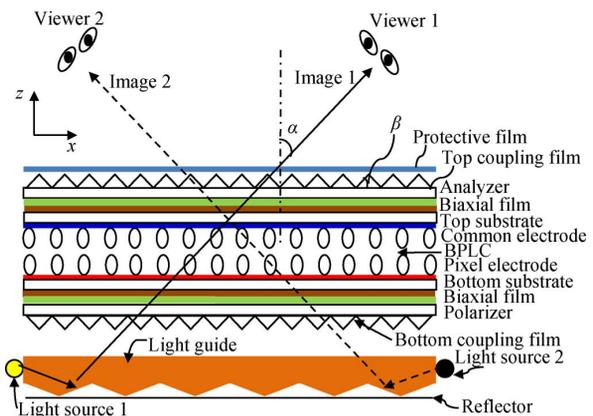
Fig. 1. Schematic of the proposed dual-view display device structure.
