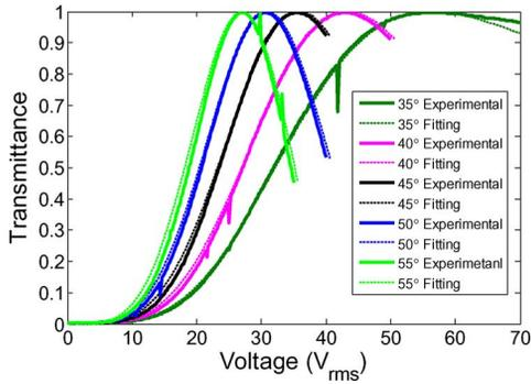
Fig. 2. VT curves of the VFS-BPLC cell at the specified incident angles. Cell gap  $d = 10 \mu\text{m}$ ,  $\lambda = 633 \text{ nm}$ , and  $T \sim 23 \text{ }^\circ\text{C}$ .
