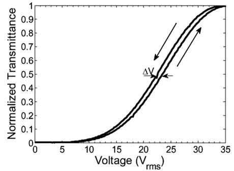
Fig. 3. Measured hysteresis of the VFS-BPLC cell at  $\theta_i = 45^\circ$ .
