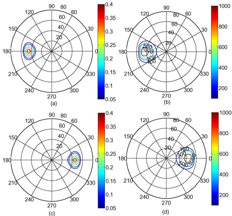
Fig. 5. Simulated (a) intensity distribution of the bright state and (b) isocontrast contour plots as the light source 2 is on; (c) intensity distribution of the bright state and (d) isocontrast contour plots as the light source 1 is on. Backlight FWHM =  $20^\circ$ ,  $\theta_i = 45^\circ$  and  $\lambda = 550$  nm.
