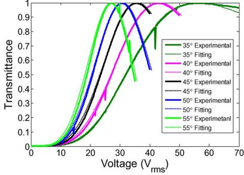
Fig. 2. VT curves of the VFS-BPLC cell at the specified incident angles. Cell gap  $d = 10 \mu\text{m}$ ,  $\lambda = 633 \text{ nm}$ , and  $T \sim 23 \text{ }^\circ\text{C}$ .
