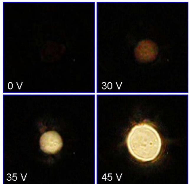
Fig. 3. (Color online) Observed images of a relatively small droplet (aperture  $\sim 140 \mu\text{m}$ ) covered by a thicker ( $\sim 30 \mu\text{m}$ ) black liquid layer.
