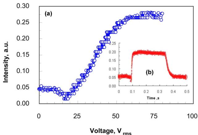
Fig. 4. (Color online) (a) Voltage-dependent transmittance and (b) the measured response time of the droplet with  $V = 45$  V<sub>rms</sub> (500 Hz) and  $\lambda = 633$  nm.
