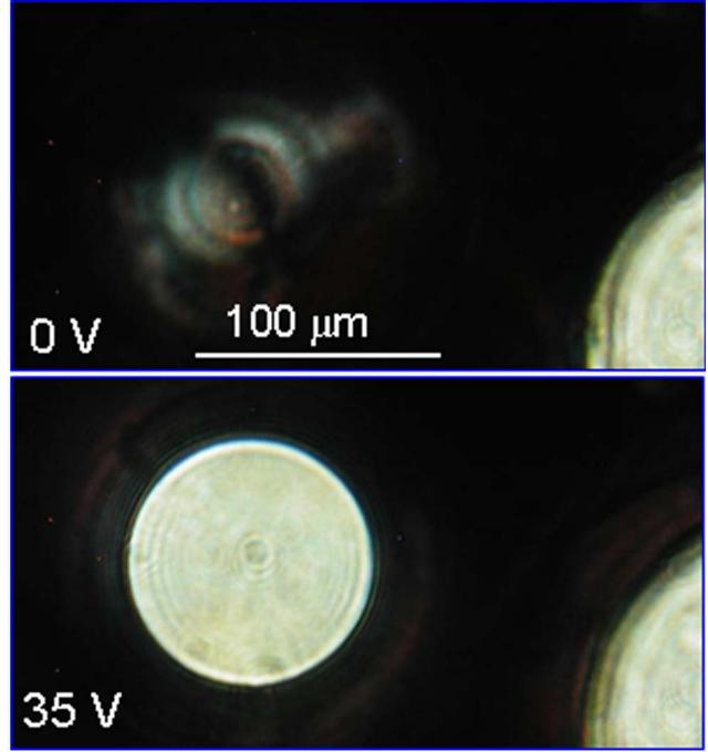
Fig. 2. (Color online) Observed images of two droplets at  $V = 0$  and  $35 \text{ V}_{\text{rms}}$  under an optical microscope with white light.
