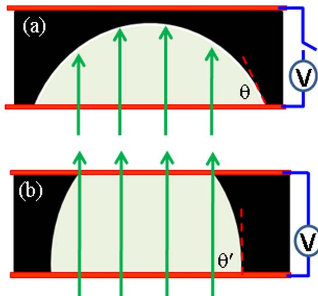
Fig. 1. (Color online) Schematic cross section of a liquid droplet cell in (a) voltage-off state and (b) voltage-on state.
